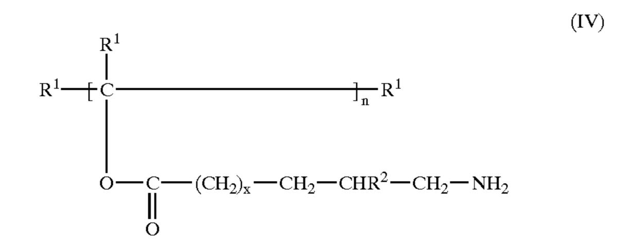
[0028] wherein each  $R^1$  is independently selected from hydrogen and  $C_{1-8}$  alkyl radicals;  $R^2$  is selected from hydrogen, methyl, ethyl, and vinyl radicals; x is an integer from 3 to about 7; and n is an integer from 2 to about 15.
