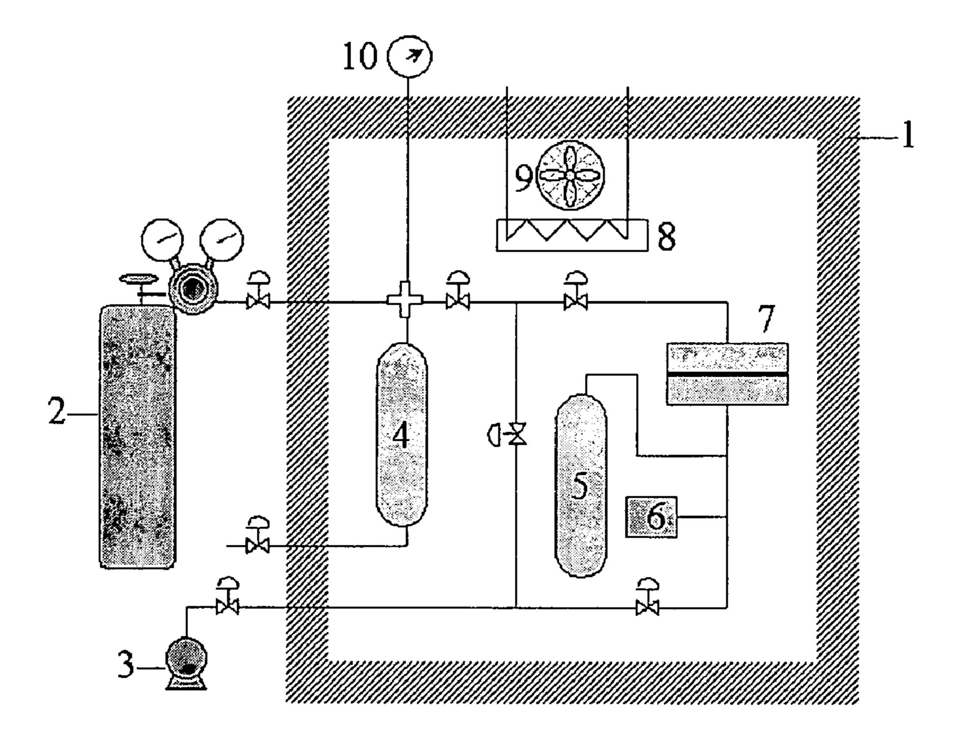
FIG. 1 Schematic of gas permeation apparatus for flat membrane films
