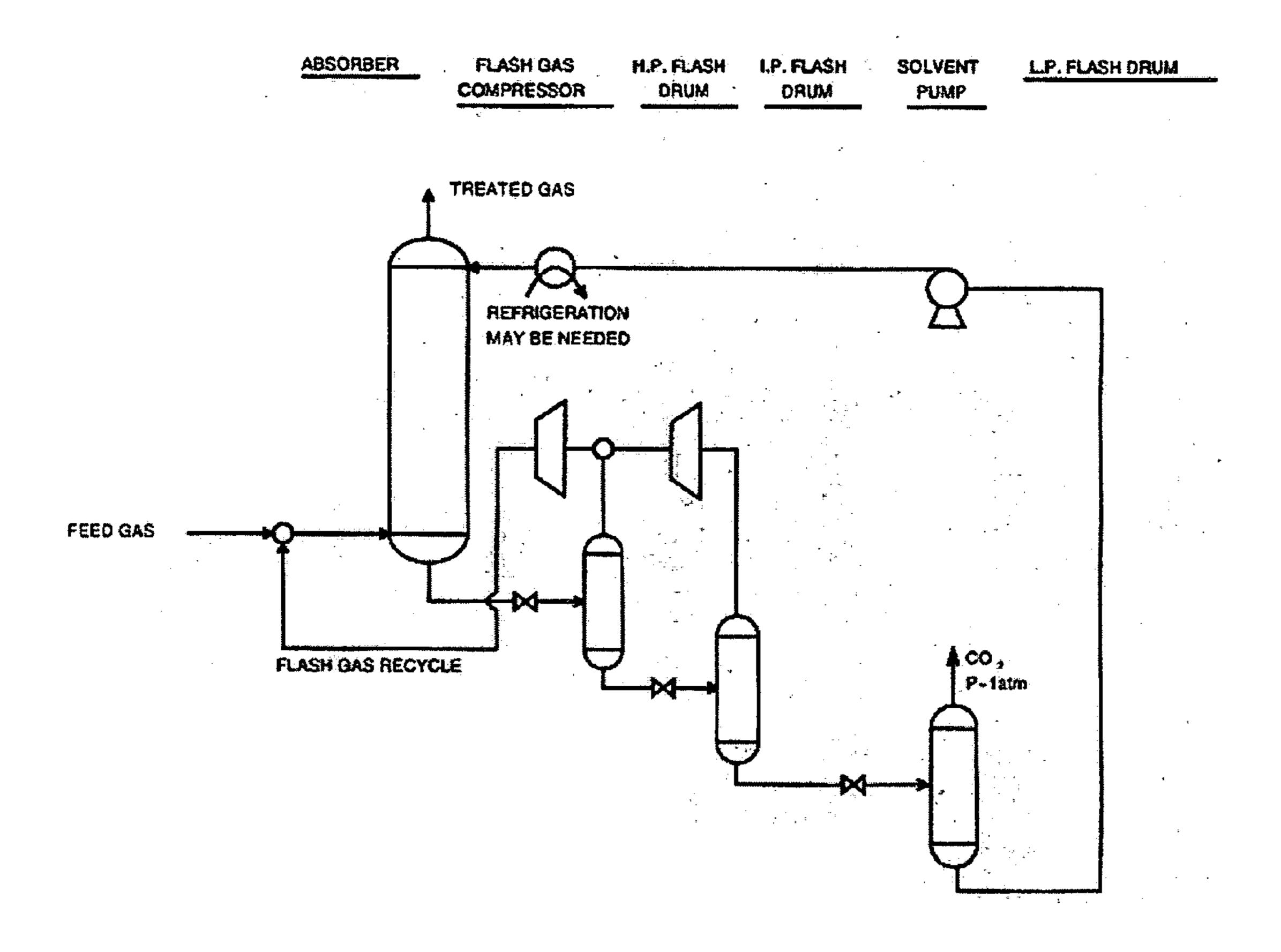
Figure 1 lonic Liquid CO<sub>2</sub> Removal Process using Flash Regeneration
