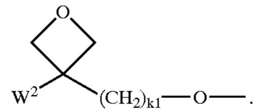
[0077] Very preferred are acrylate and oxetane groups. Oxetanes produce less, shrinkage upon polymerization (cross-linking), which results in less stress development within films, leading to higher retention of ordering and fewer defects. Oxetane cross-linking also requires cationic initiator, which unlike free radical initiator is inert to oxygen.
