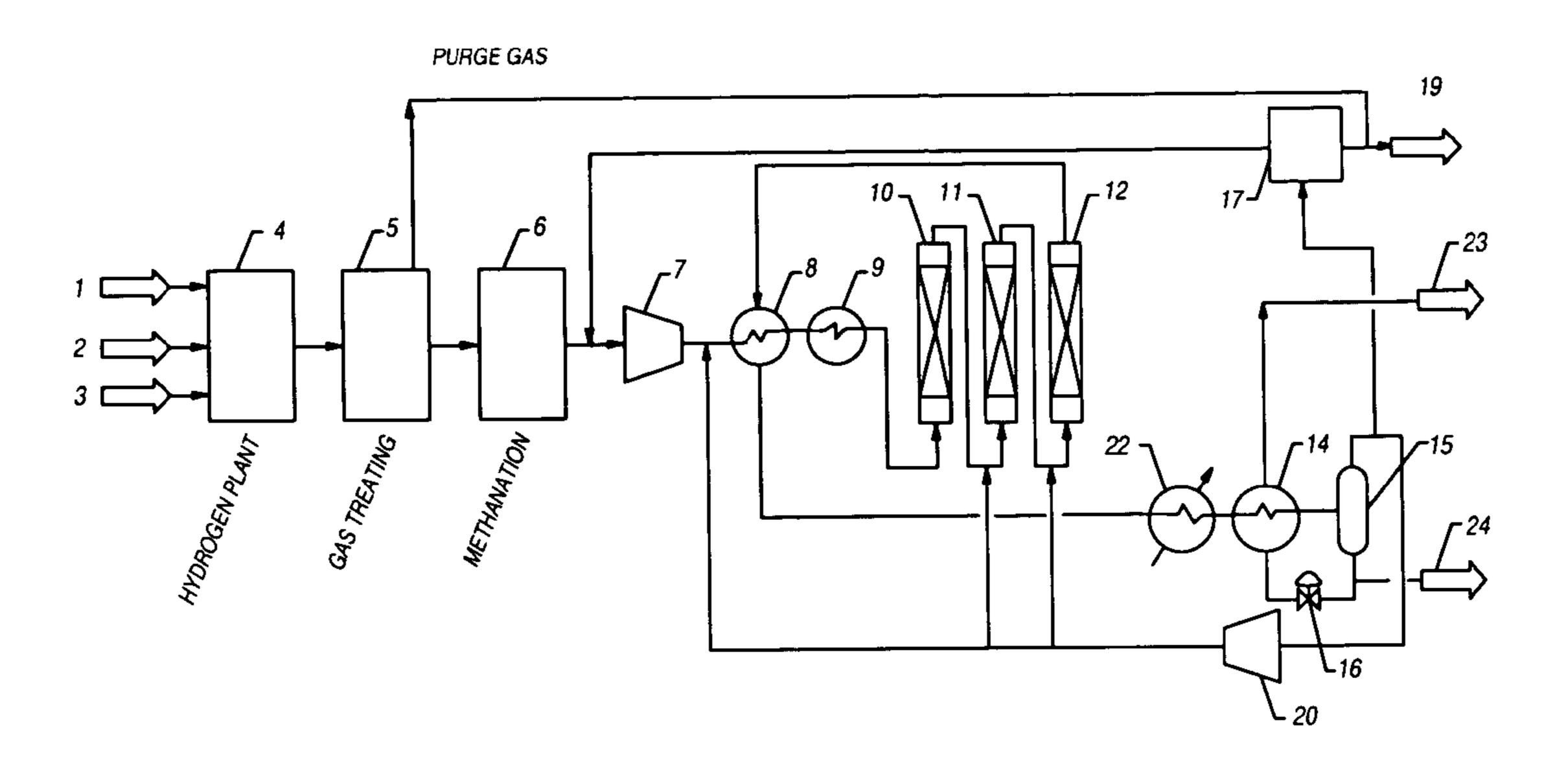
Figure 3 Flow Diagram with Pure Ammonia Output For Industrial Applications
