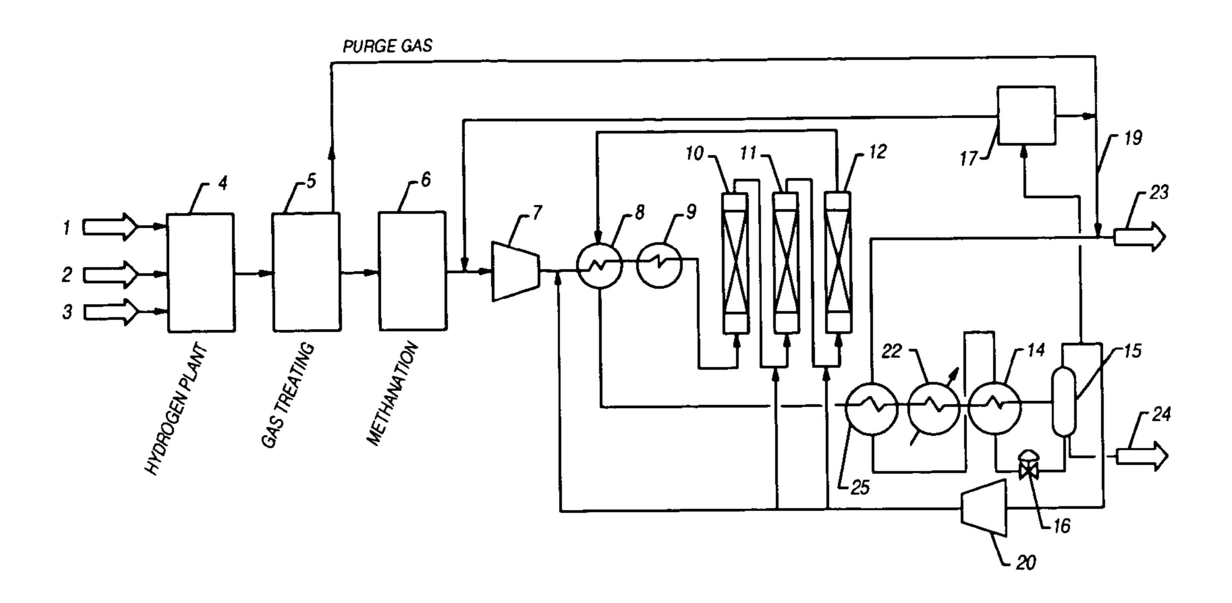
Figure 2 Flow Diagram with Hot Ammonia Gas Output For SCR Applications
