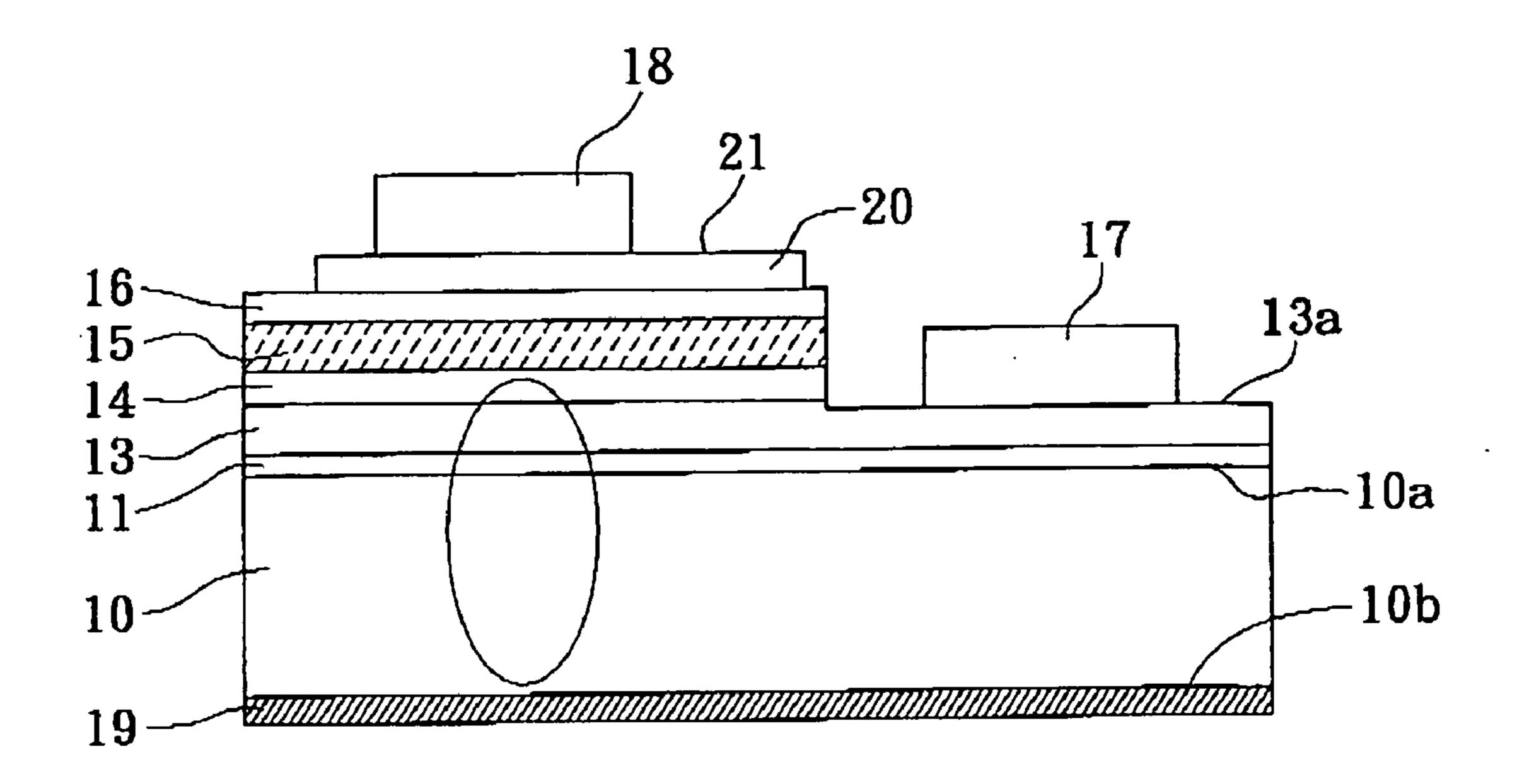
FIG. 5 Au/Ni 201 **--161** P + -GaN-based P-AIGaN/GaN DBR -151 -141 InGaN/GaN MQW n-GaN 131 -111 GaN(buffer layer) Sapphire(substrate) 101 <u>—191</u> metal Reflector
