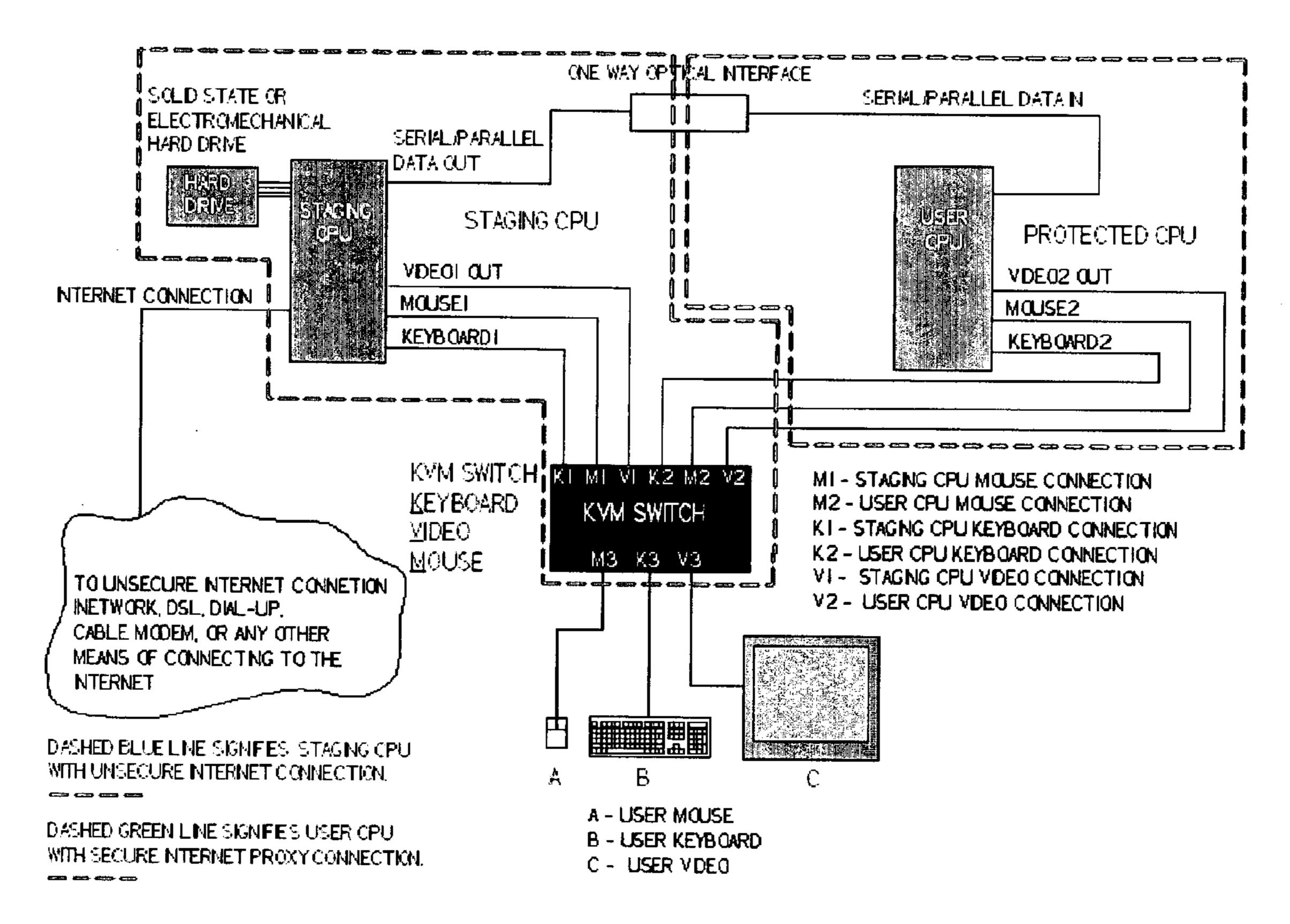
NOTE: STAGING CPUICAN BE A PHYSICAL COMPUTER OR A CPUICARD PLACED INSIDE USER CPUI
