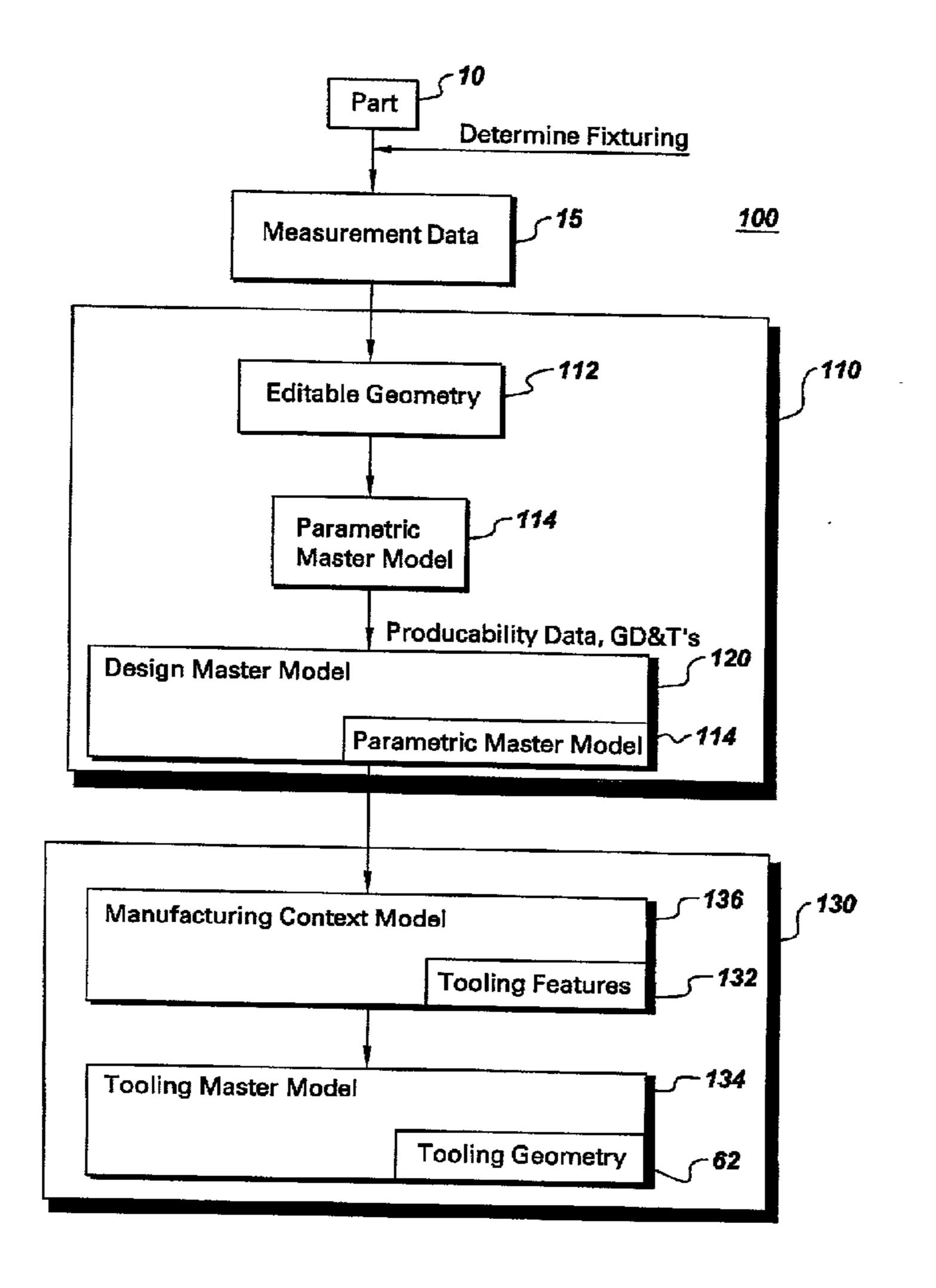
Fig. 1 Part Determine Fixturing 100 Measurement Data 110 Editable Geometry Parametric Master Model Producability Data, GD&T's 120 Design Master Model Parametric Master Model -136 Manufacturing Context Model **Tooling Features** -134 Tooling Master Model **Tooling Geometry**
