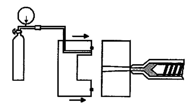
2. Injection into the cavity under counter-pressure
