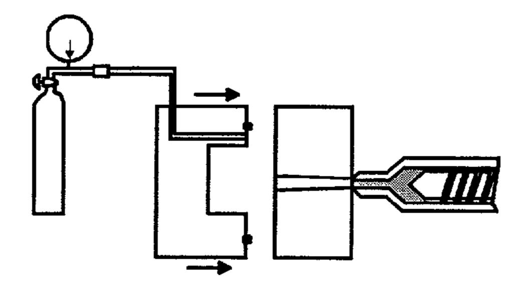
2. Injection into the cavity under counter-pressure
