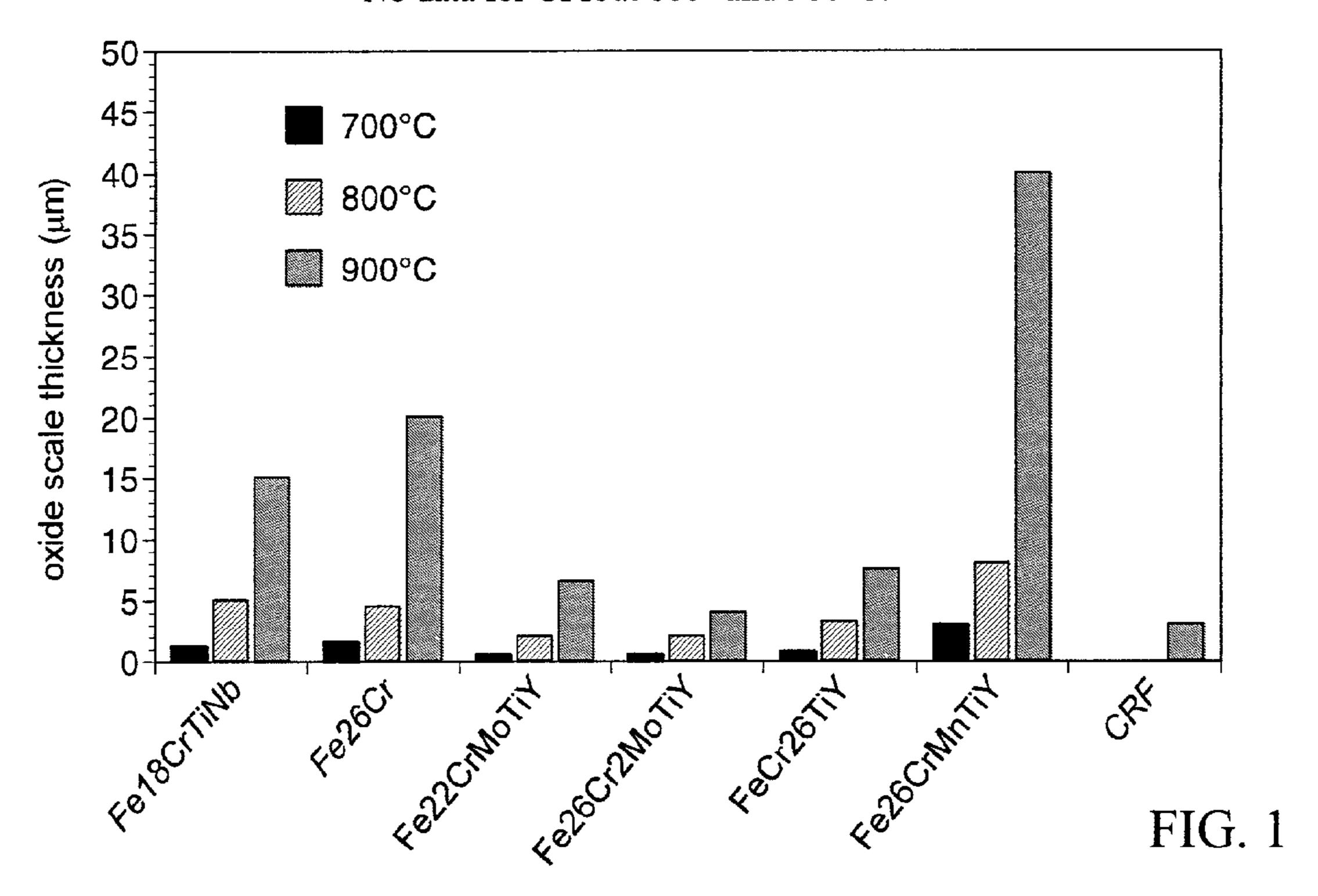
Comparison – oxide scale thickness, exposure air. Fe26Cr (446) start peeling at 800°C; oxide scale falls off at 900°C
