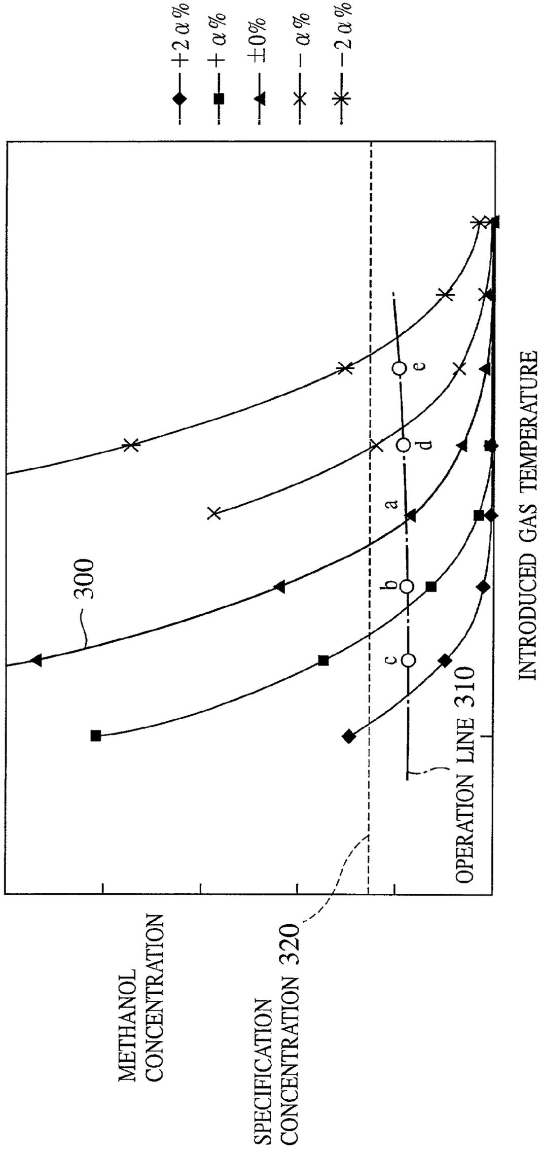
DIAGRAM OF METHANOL CONCENTRATION AND INTRODUCED GAS TEMPERATURE
