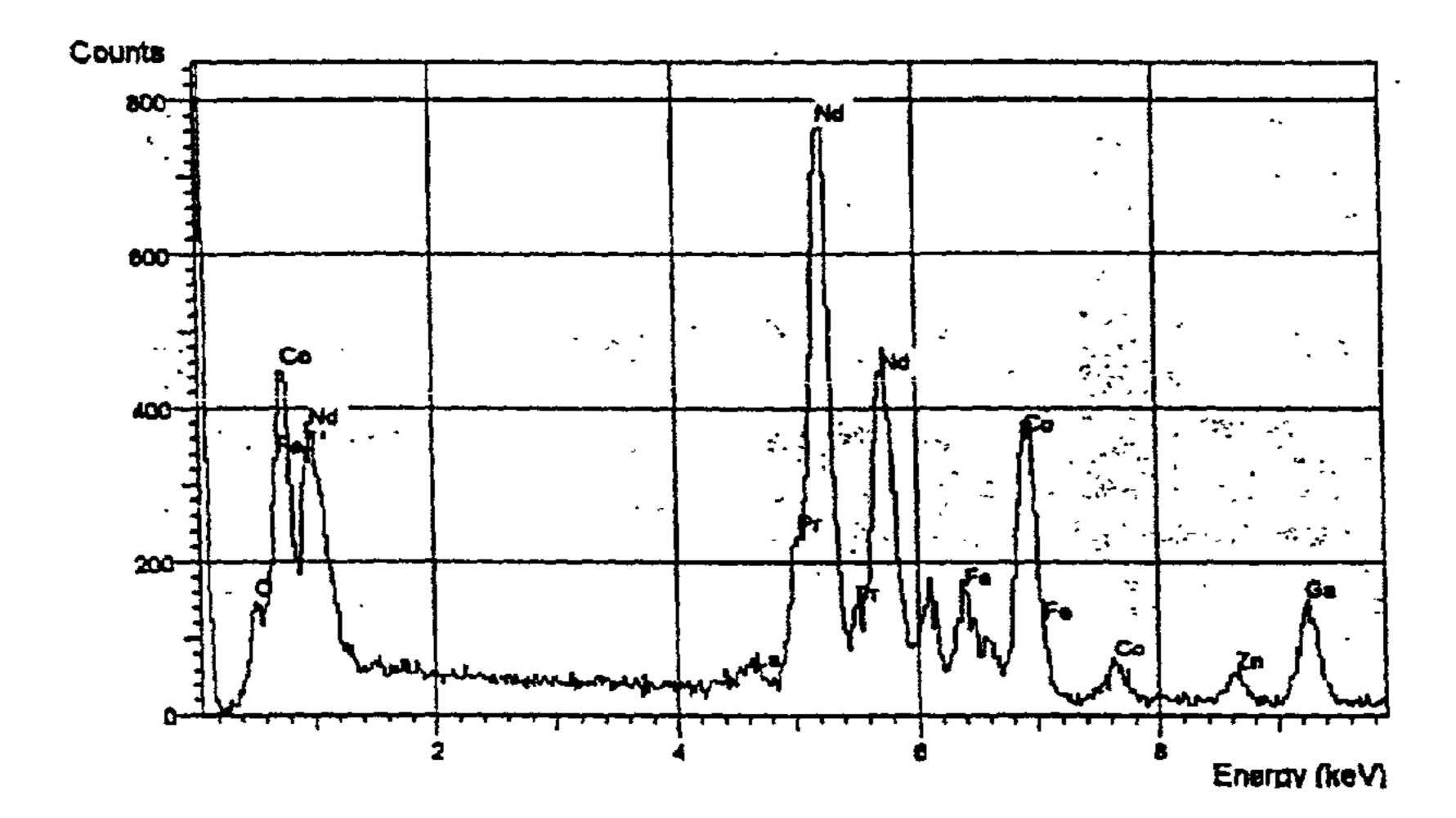
EDX spectrum of the particle amorphous phase located at matrix grain boundaries. Chemical composition of this phase: O - 38.8at.%, Nd - 31.4at.%, Co - 14.2at.%
