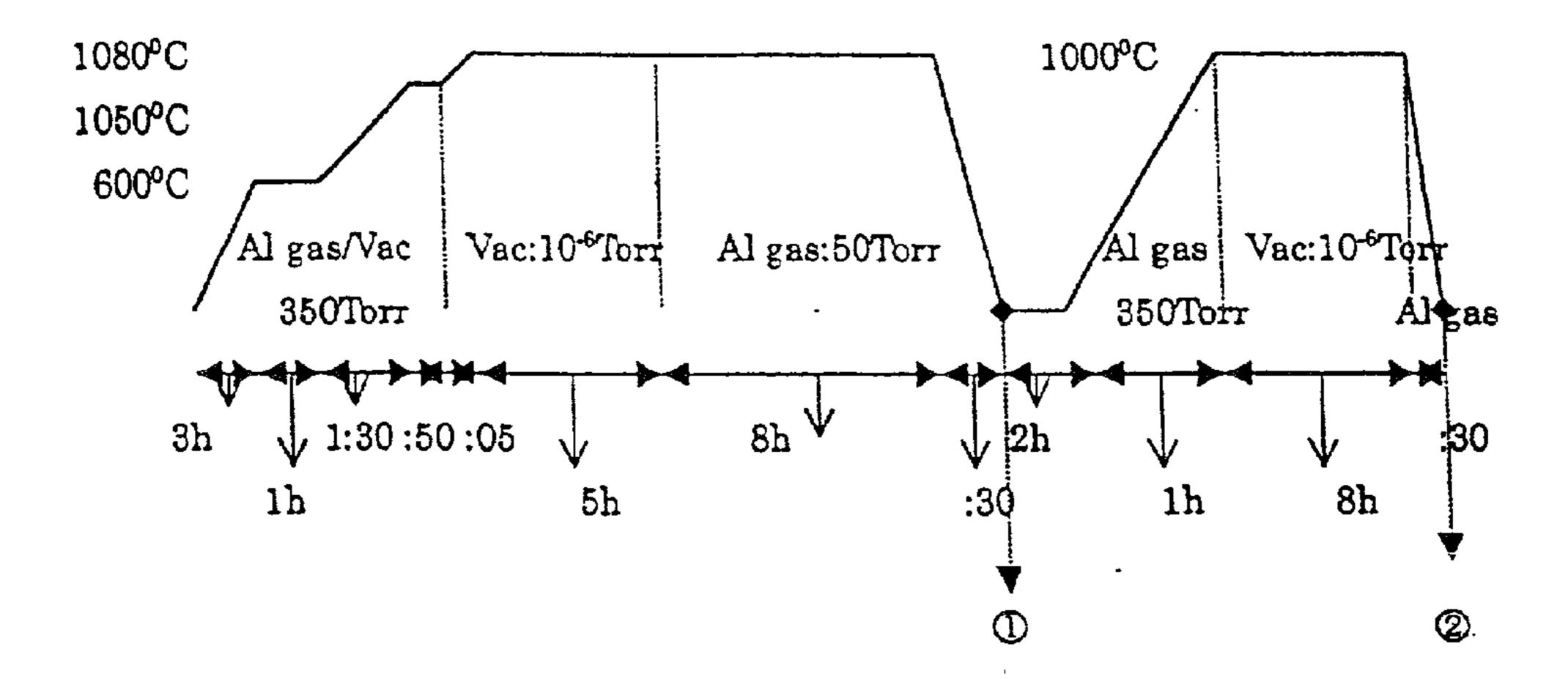
sintering and crystalization process
