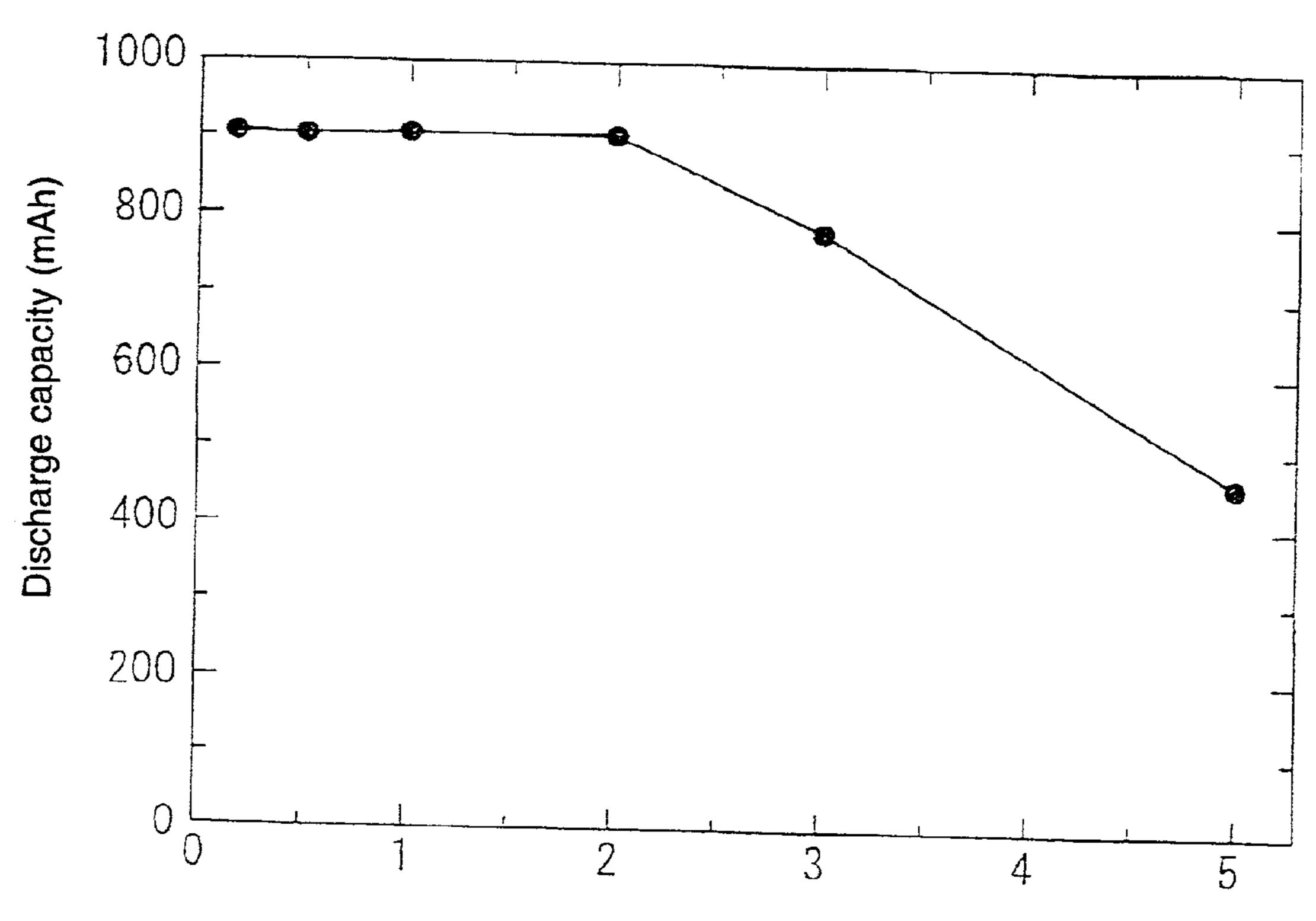
Time from injection of electrolyte to initiation of charging (h)
