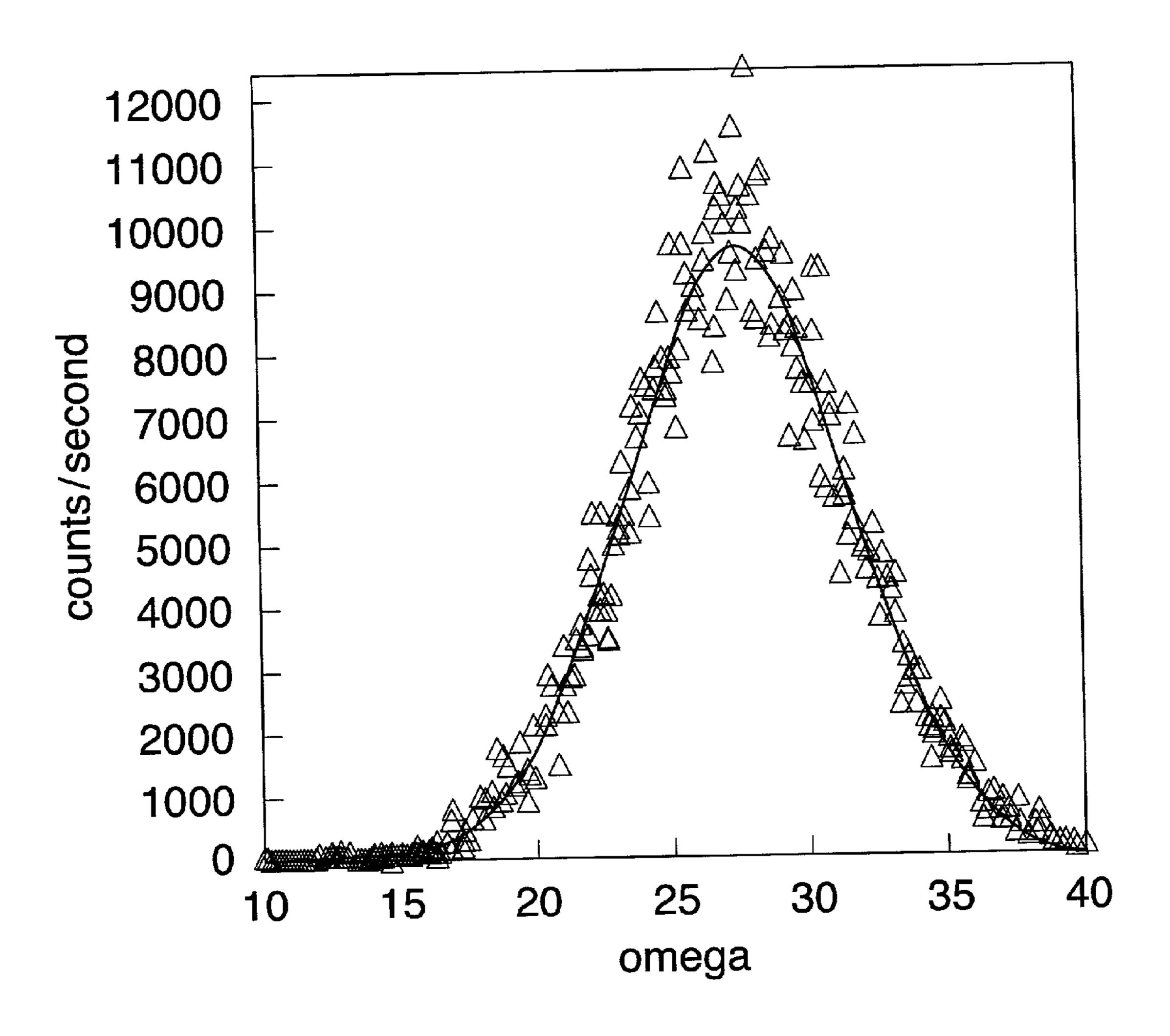
Ni-13at%Cr-0.03at%Mg alloy Annealing Temperature = 1200°C
