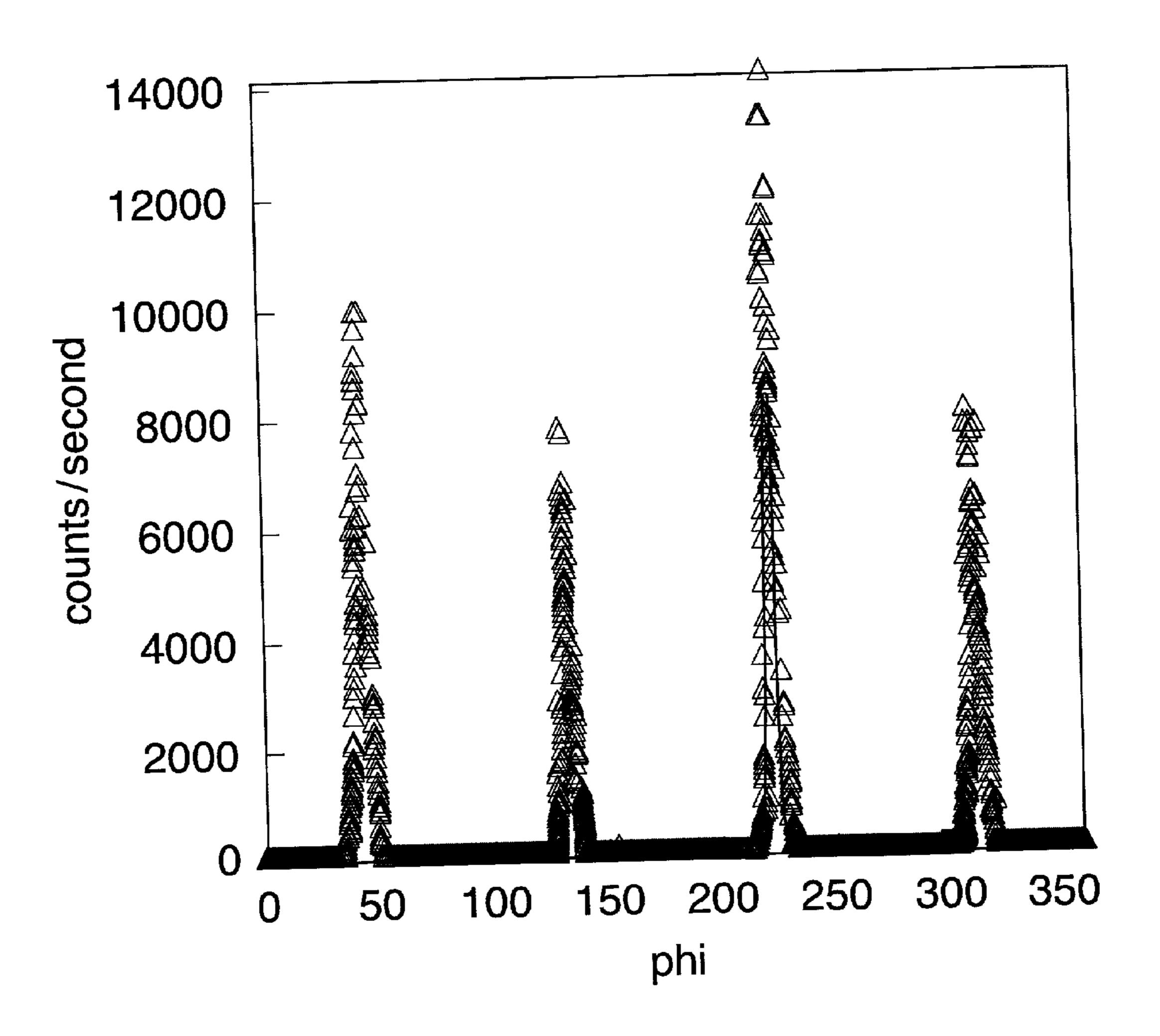
Ni-9at%W alloy Annealing Temperature = 1400°C
