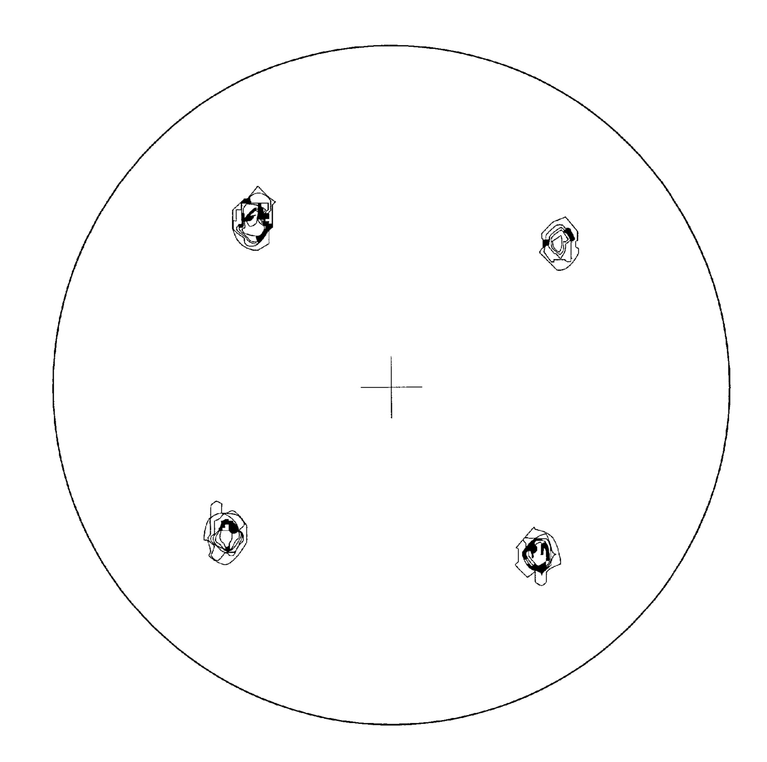
Ni-13at%Cr-0.03at%Mg alloy Annealing Temperature = 1200°C
