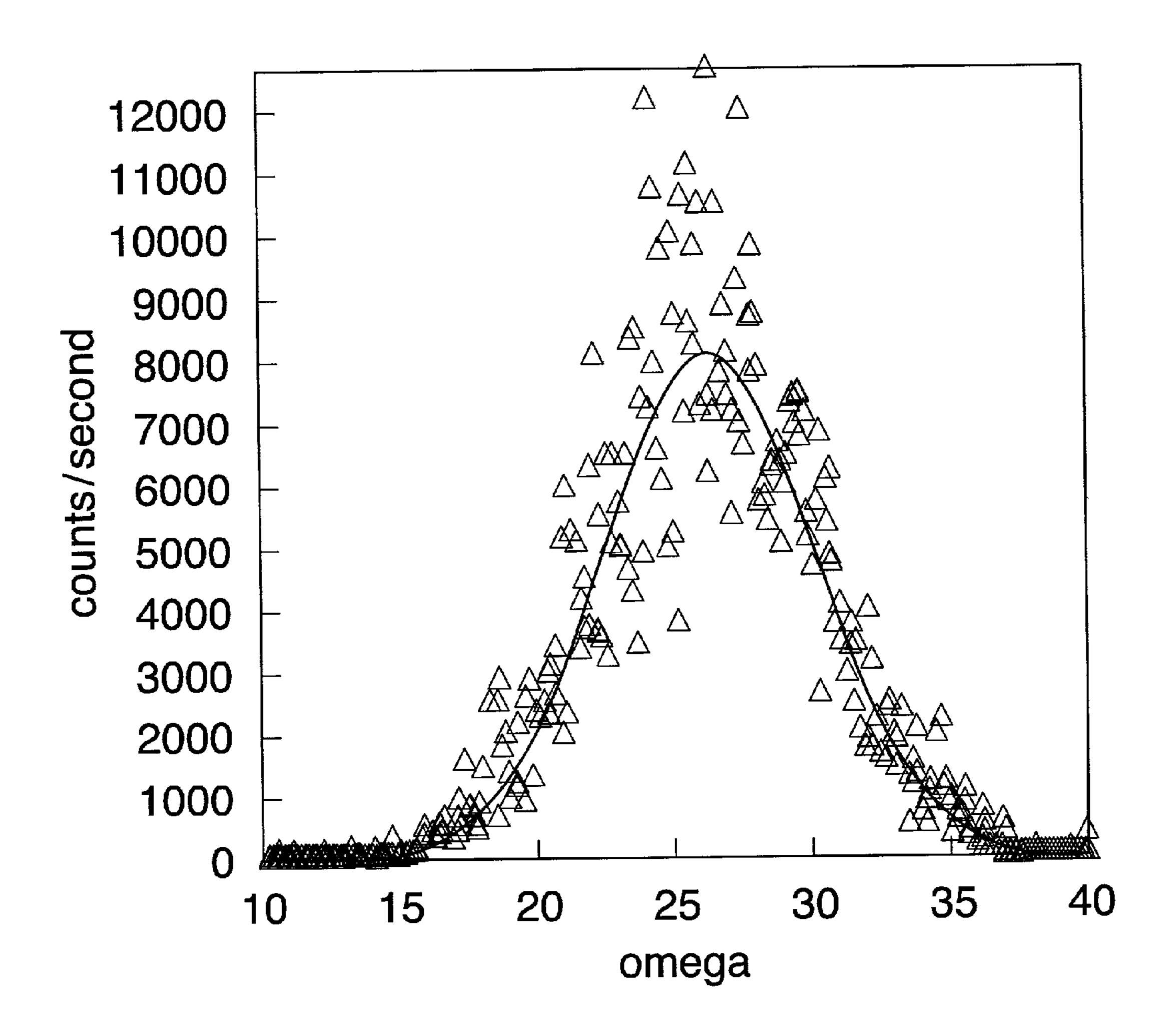
Ni-9at%W-0.03at%Mg alloy Annealing Temperature = 1200°C
