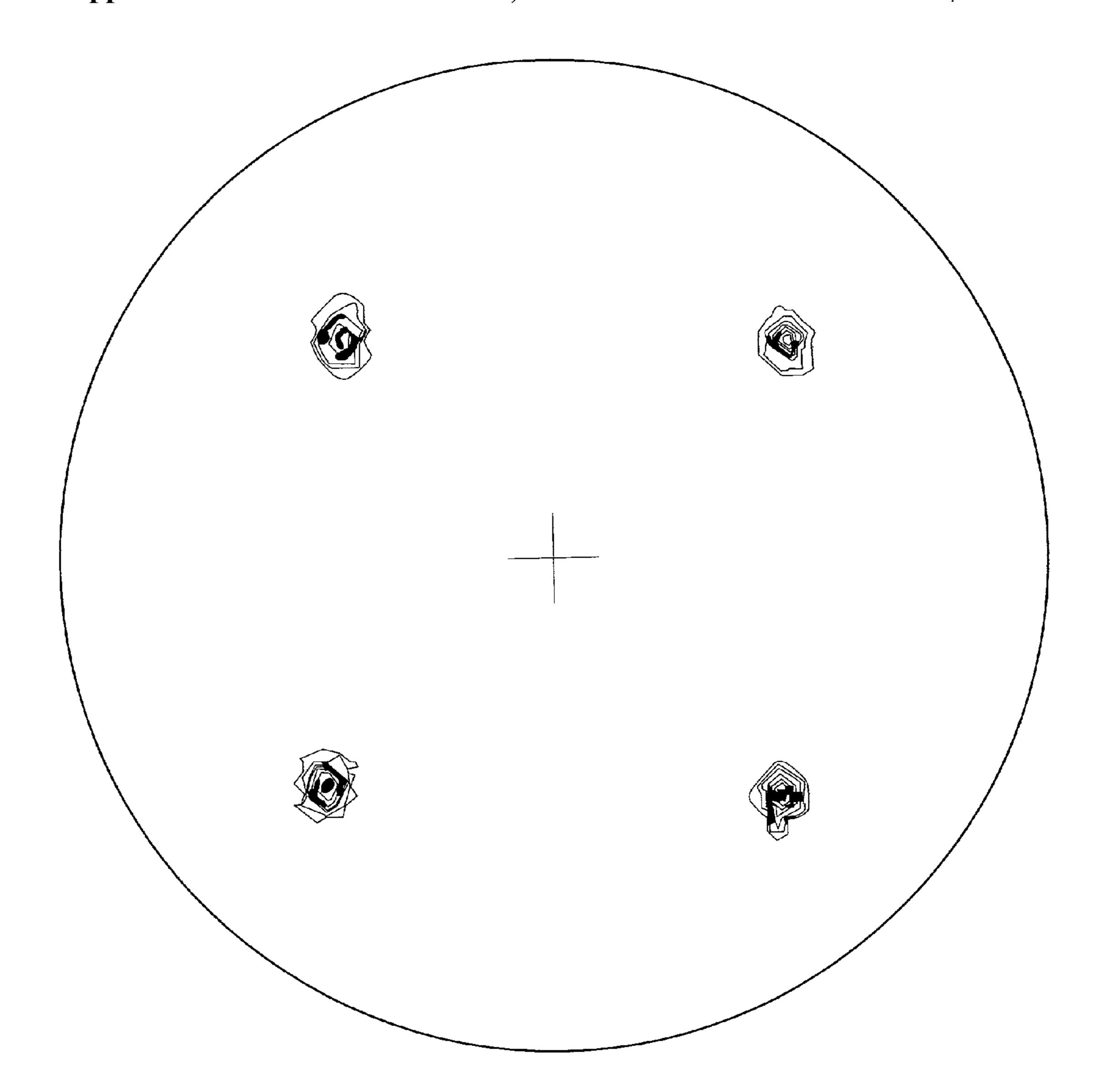
Ni-9at%W alloy Annealing Temperature = 1400°C
