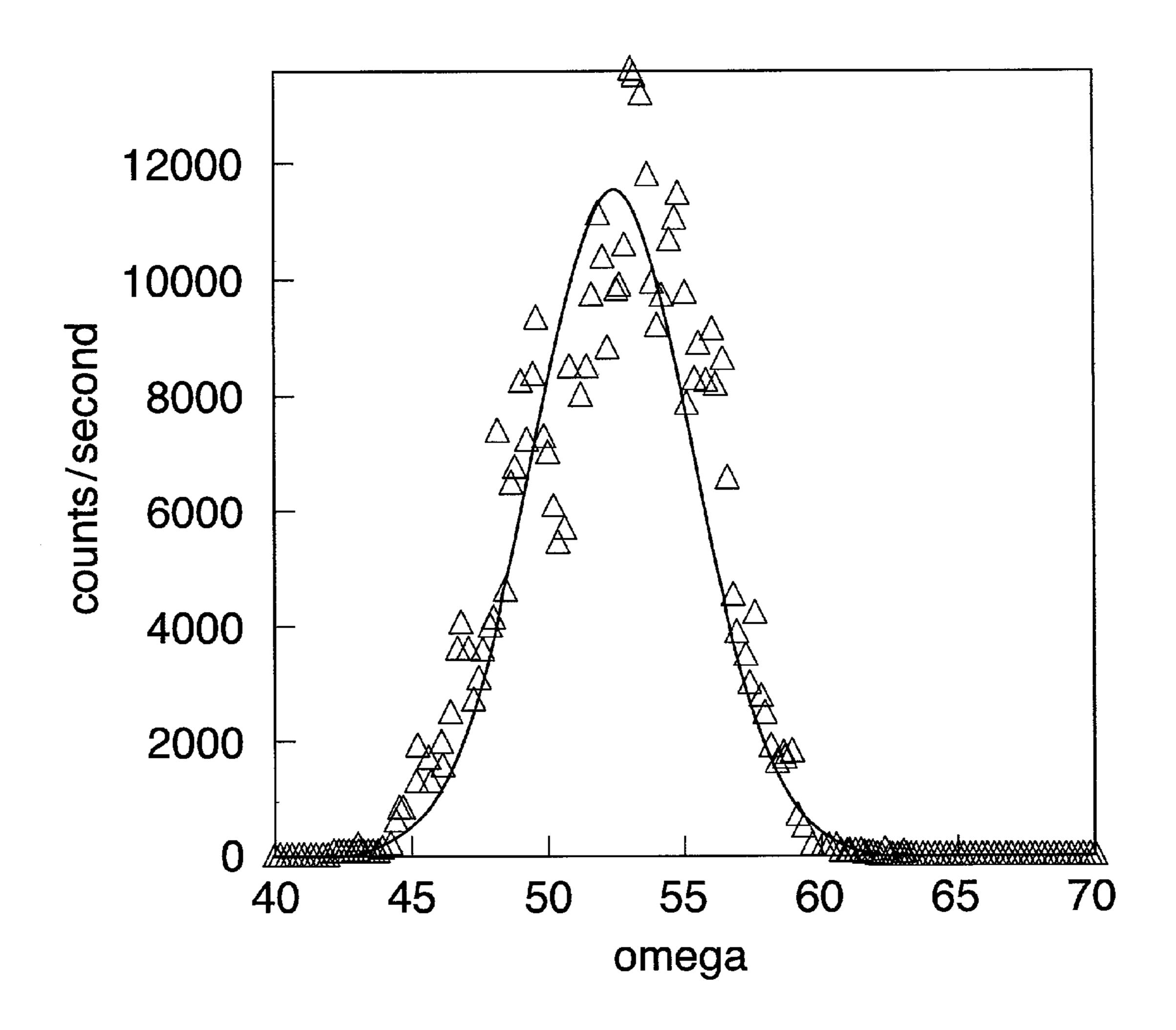
Ni-13at%Cr-0.03at%Mg alloy Annealing Temperature = 1400°C
