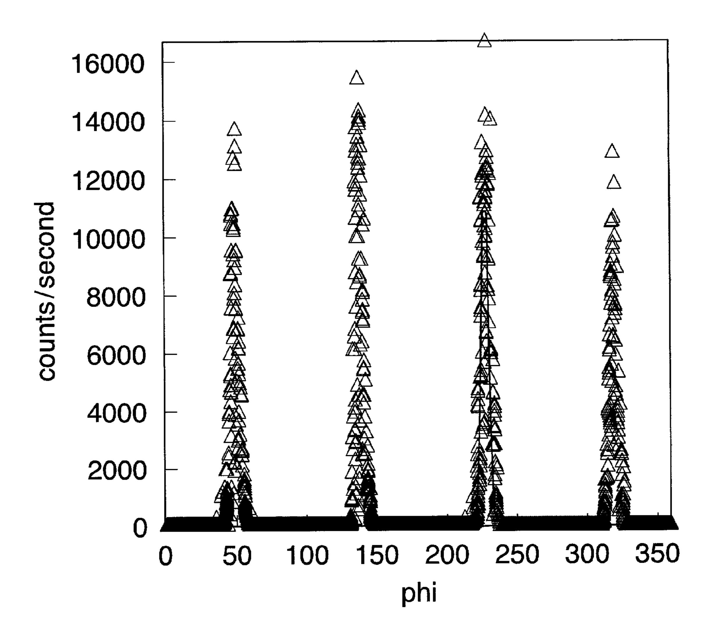
Ni-9at%W-0.03at%Mg alloy Annealing Temperature = 1400°C
