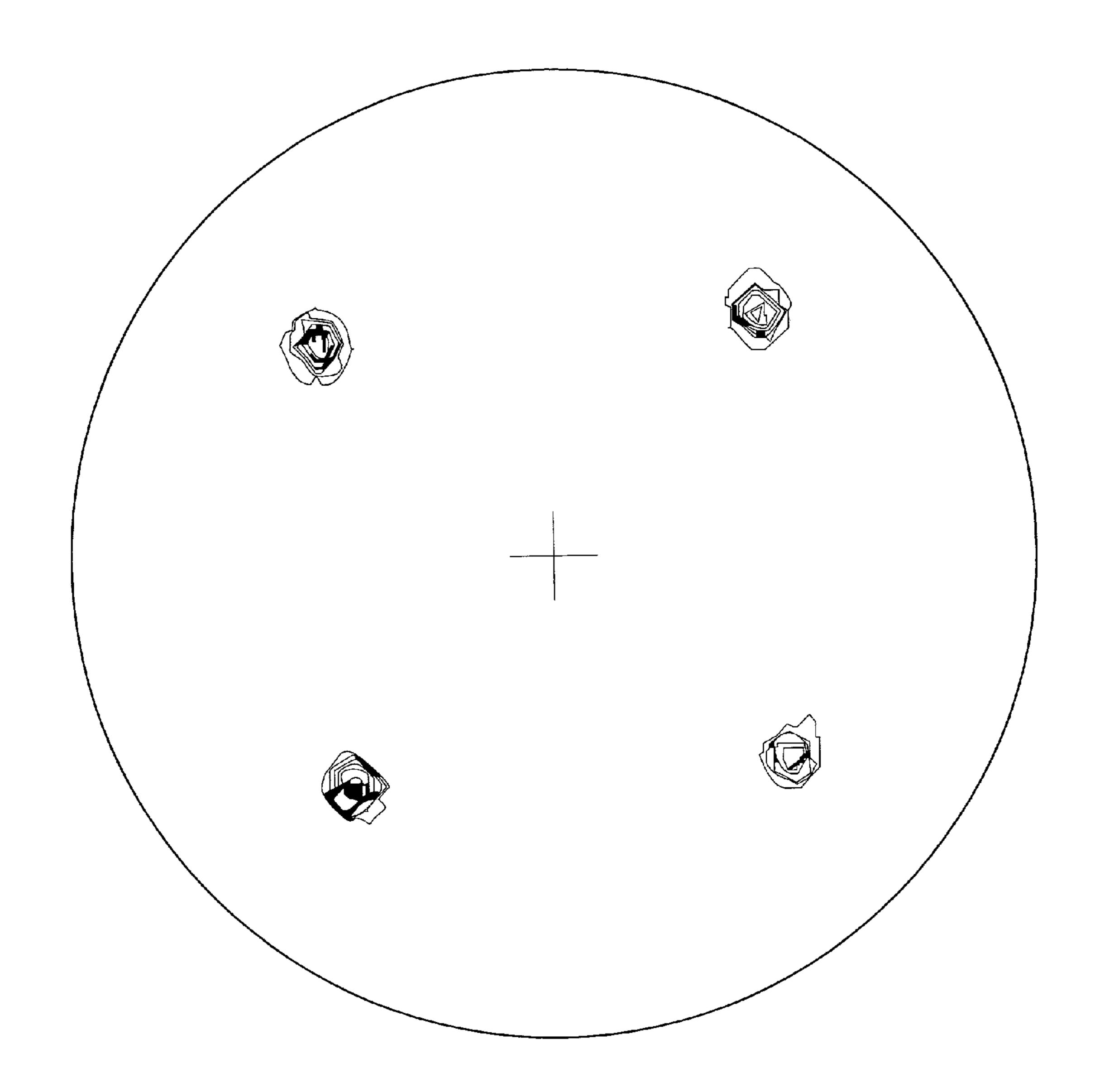
Ni-9at%W-0.03at%Mg alloy Annealing Temperature = 1400°C
