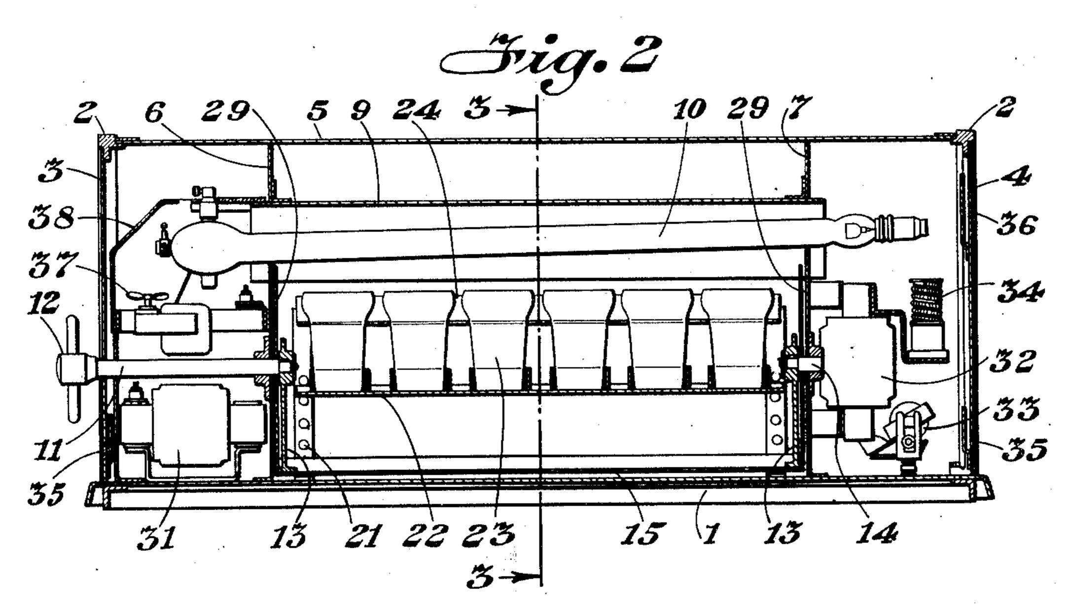
INVENTOR Otto J. Moehler BY ATTORNEY APPARATUS FOR STERILIZING ARTICLES BY ULTRAVIOLET RADIATION
