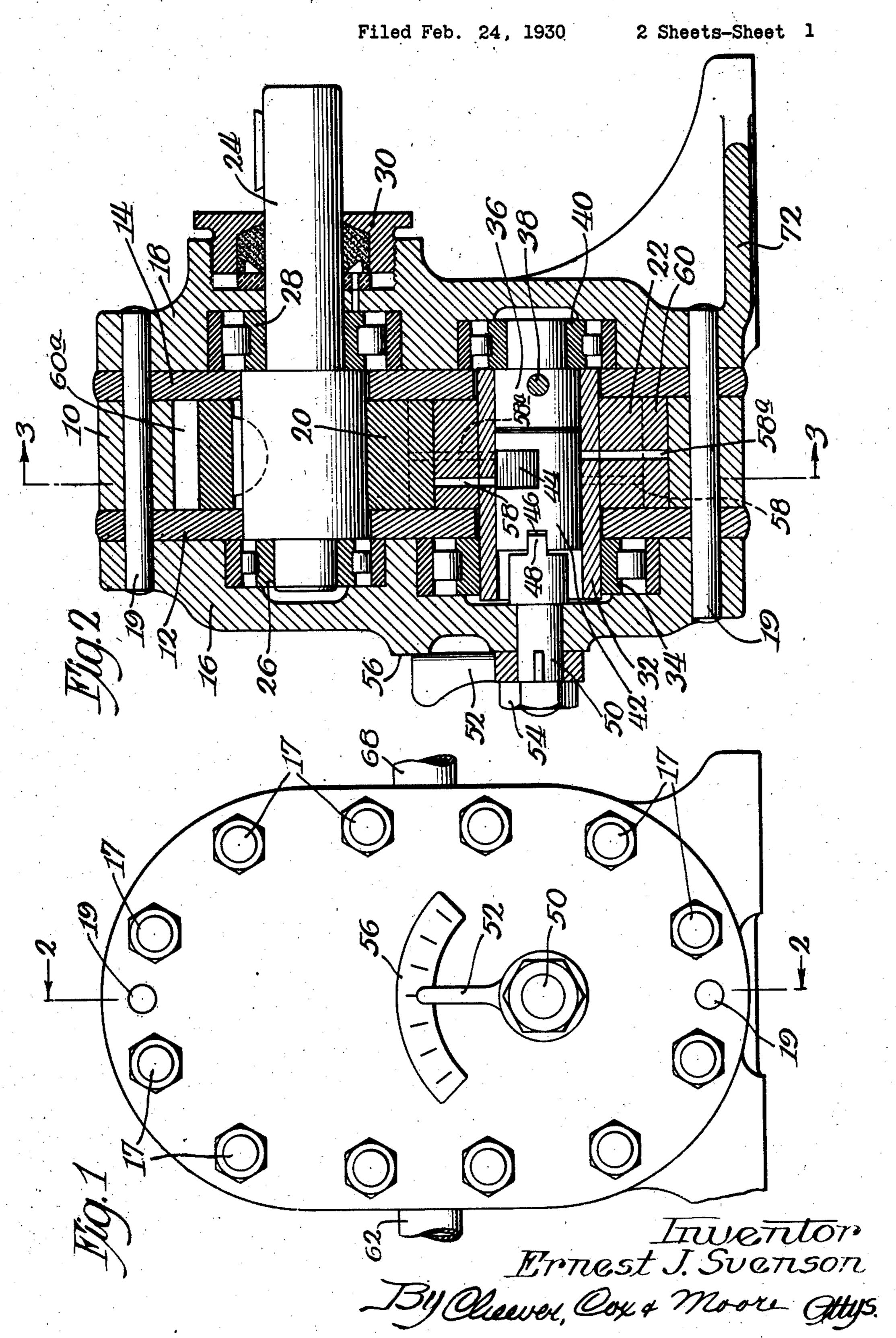
ADJUSTABLE DISPLACEMENT GEAR PUMP
