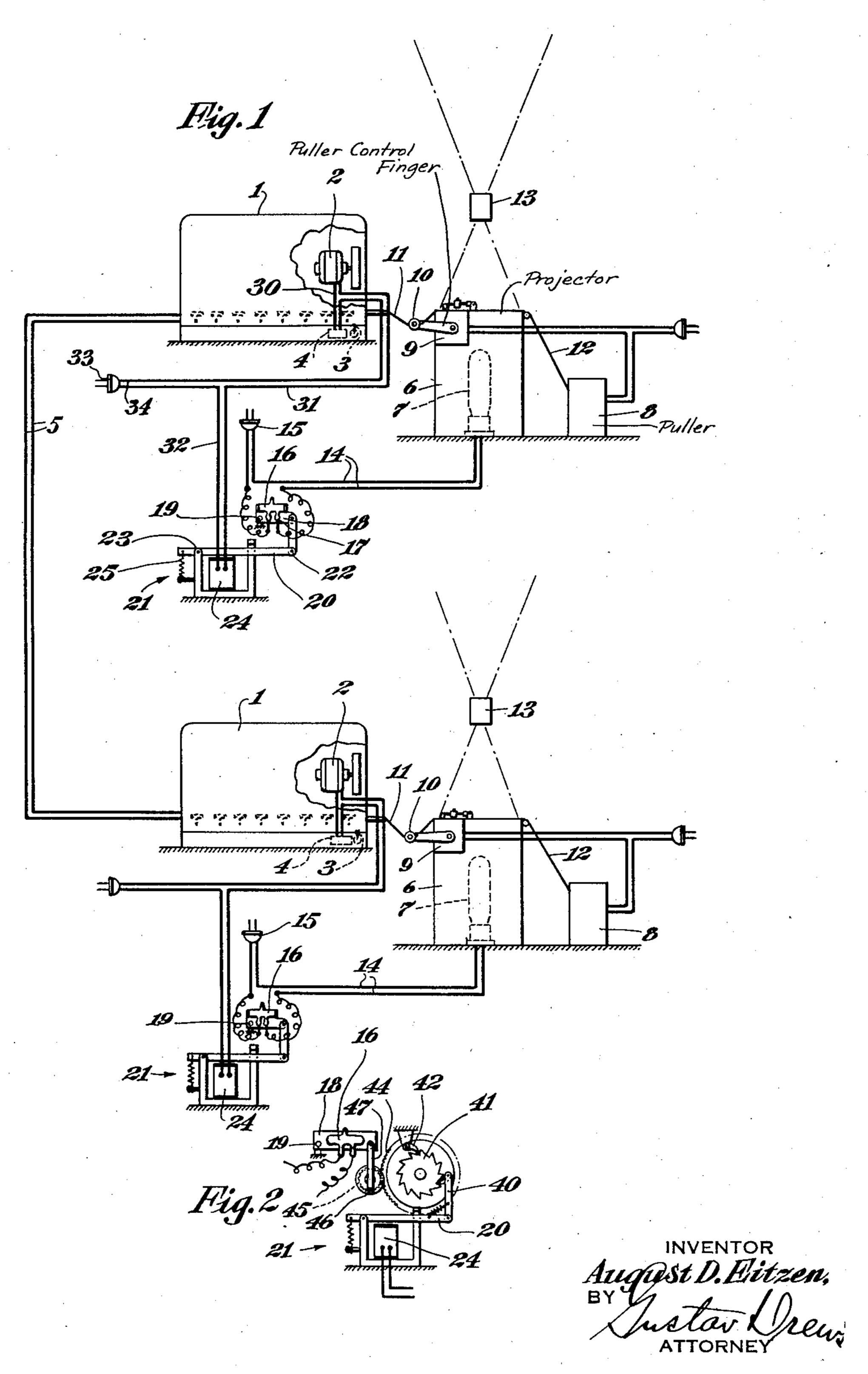
LAMP CONTROL MECHANISM FOR MESSAGE TRANSMITTING SYSTEMS
