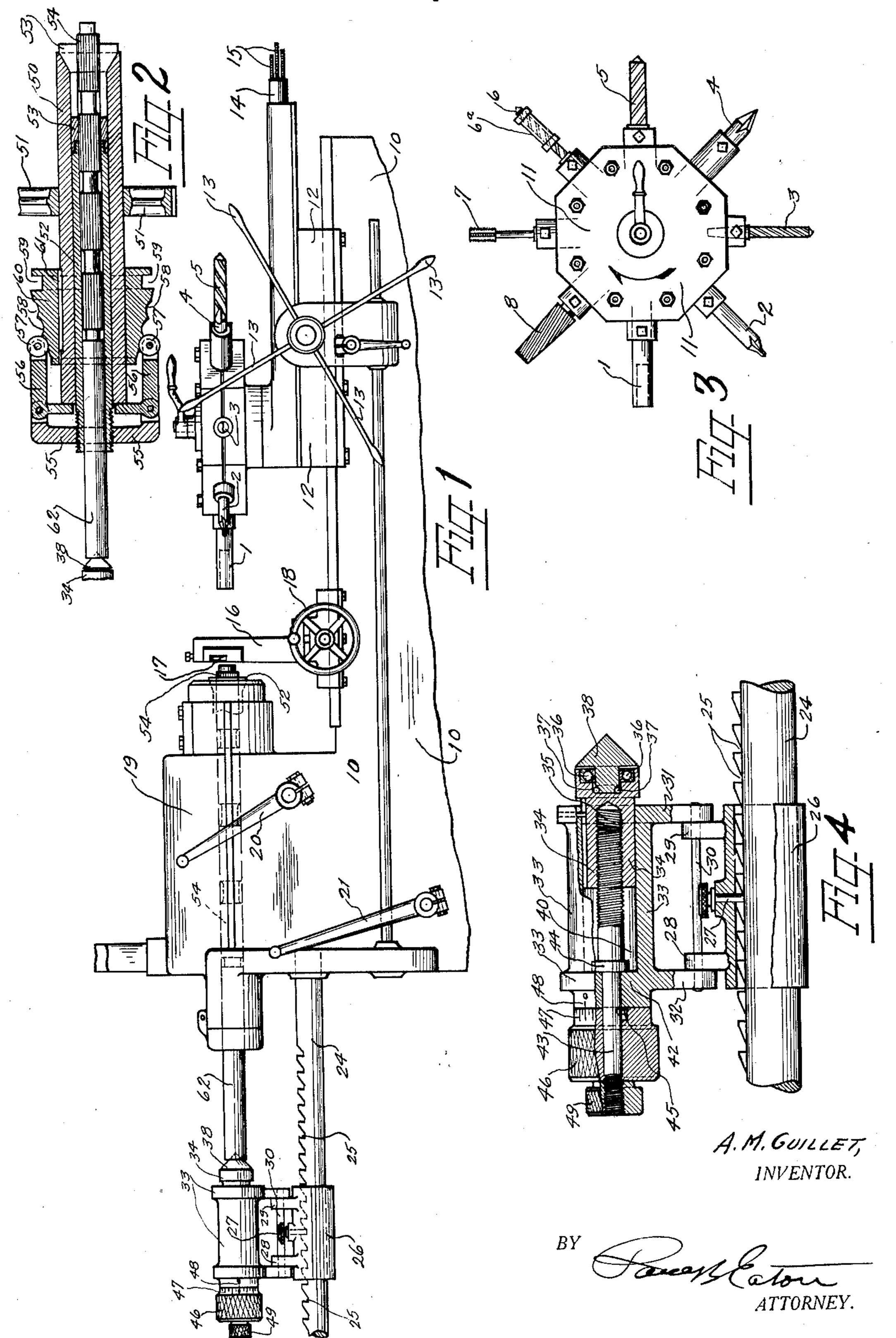
METHOD OF JOINING SECTIONS OF ROLLS TOGETHER
