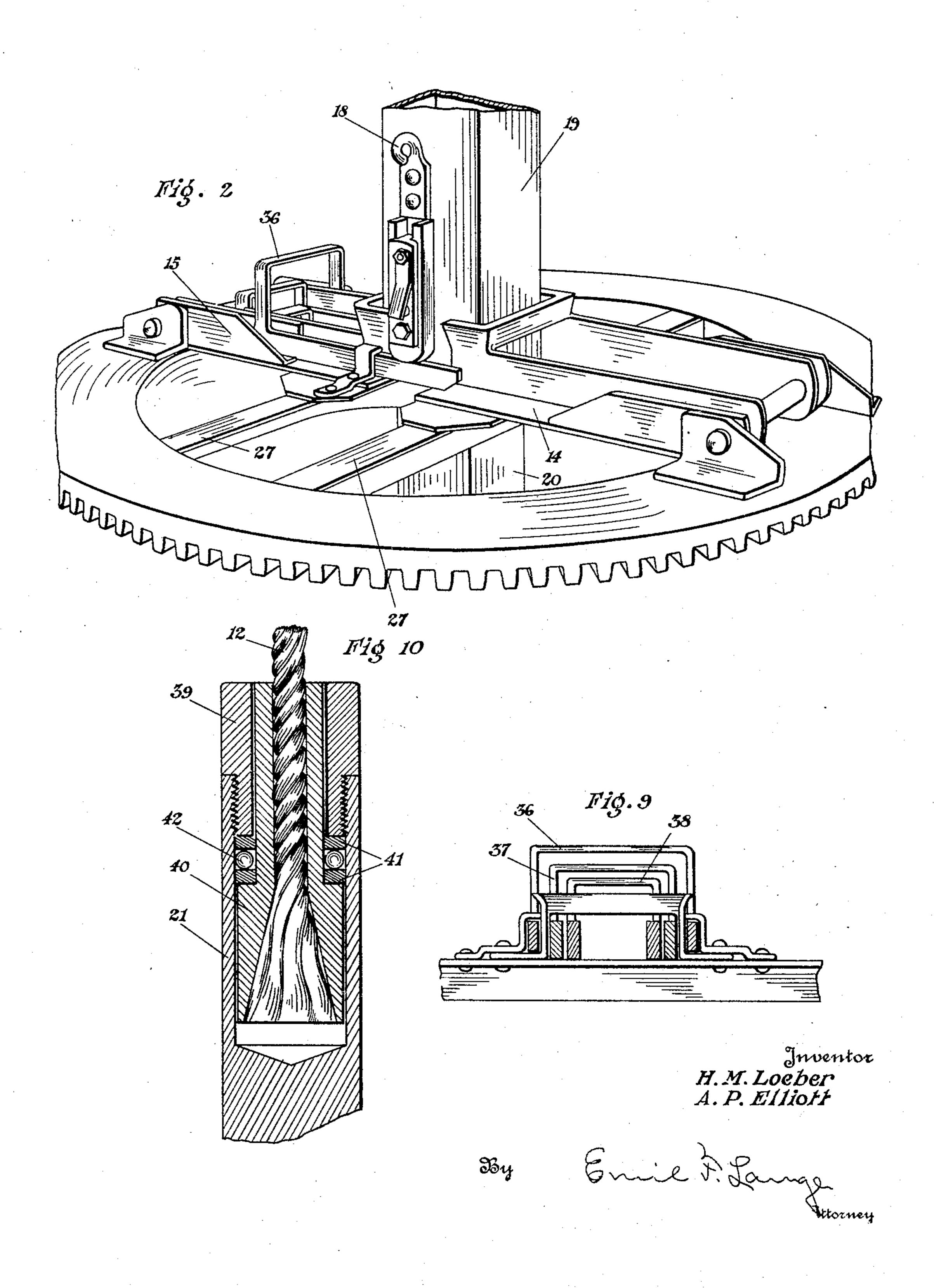
TELESCOPING BORING BAR FOR EARTH BORING MACHINES
