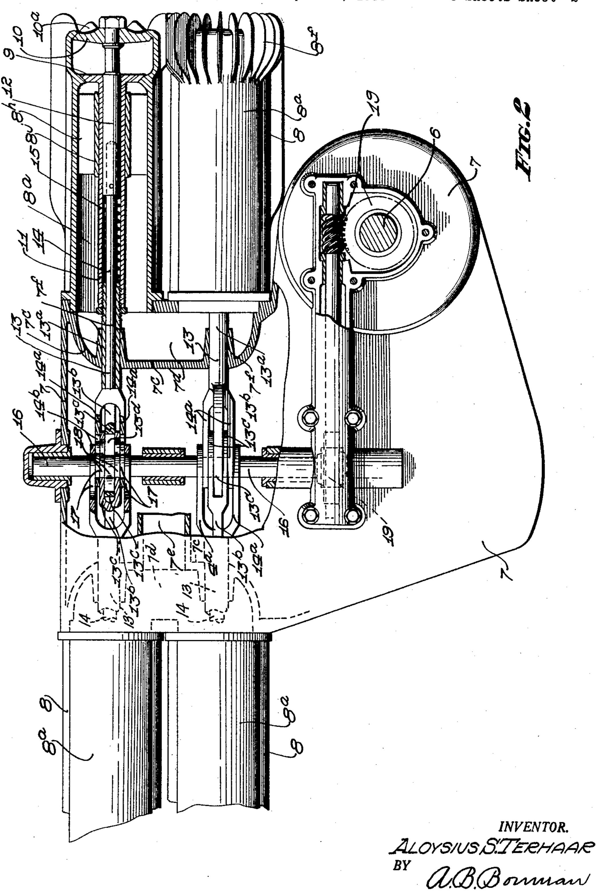
INTERNAL COMBUSTION ENGINE Filed April 9, 1930 3 Sheets-Sheet 3
