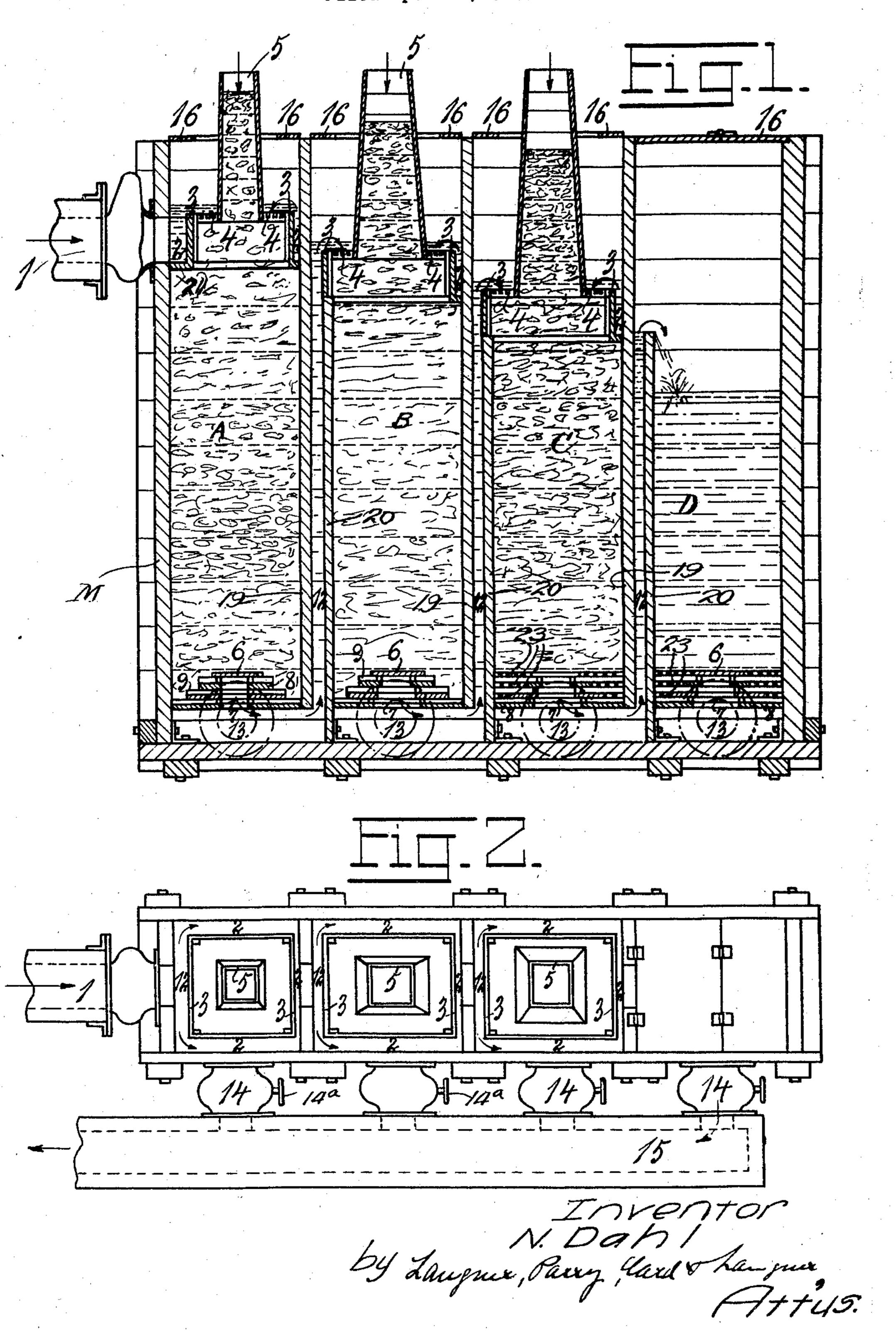
PROCESS AND APPARATUS FOR PRODUCING COOLING LIQUIDS
