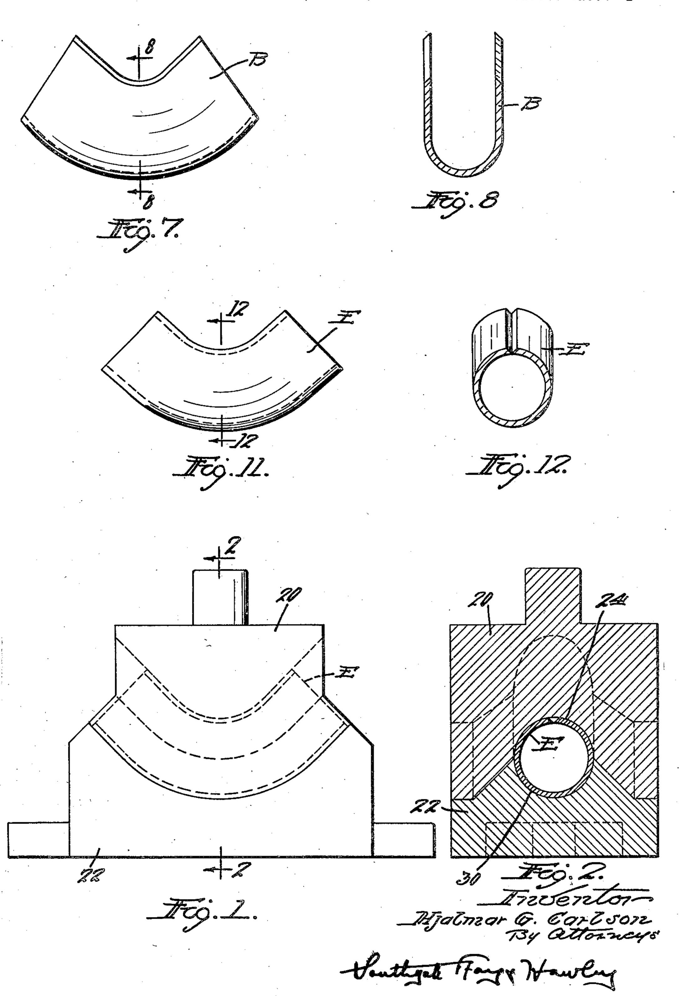
DIES AND METHOD FOR CLOSING PRESSED METAL PIPE FITTINGS
