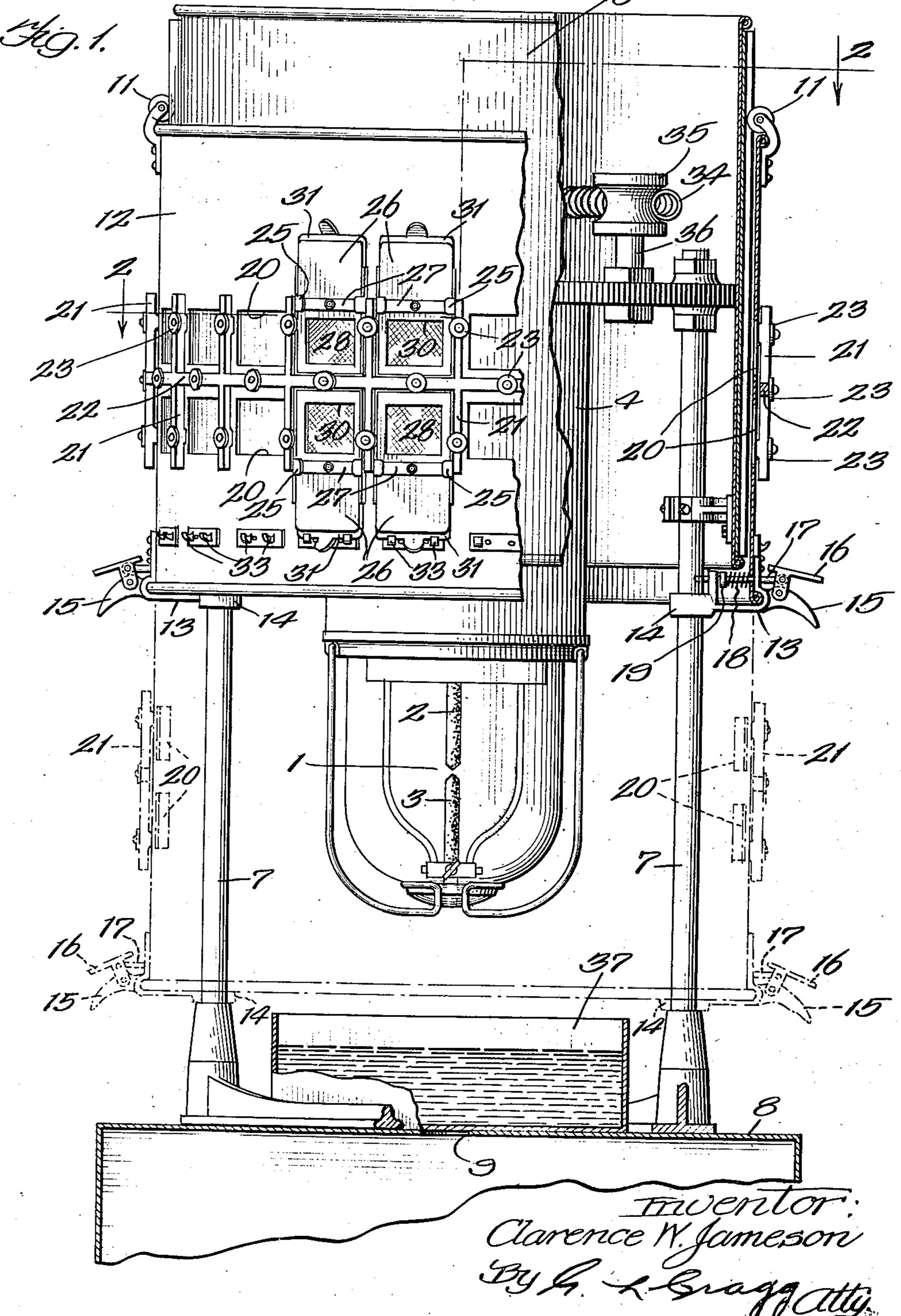
APPARATUS FOR TESTING THE FADING ACTION OF LIGHT
