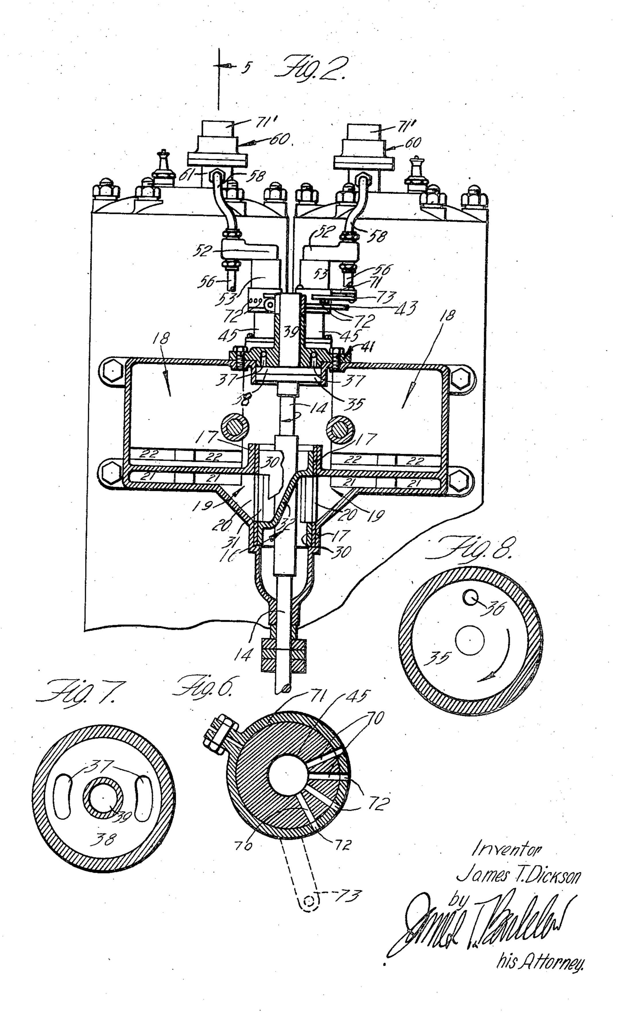
J. T. DICKSON. INJECTION MECHANISM FOR INTERNAL COMBUSTION ENGINES.
