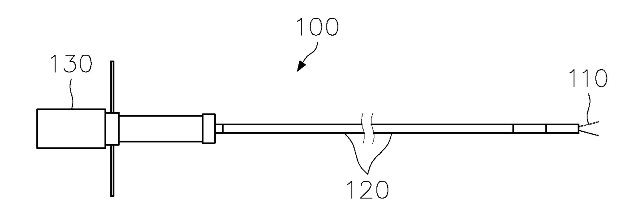
**OPENING MACHING APPARATUS FOR** HEAT TRANSFER TUBE, METHOD OF FORMING OPENING IN TUBE WALL OF HEAT TRANSFER TUBE USING SAME, AND METHOD OF REMOVING FOREIGN MATERIAL THROUGH SAME OPENING OF SAME HEAT TRANSFER TUBE
