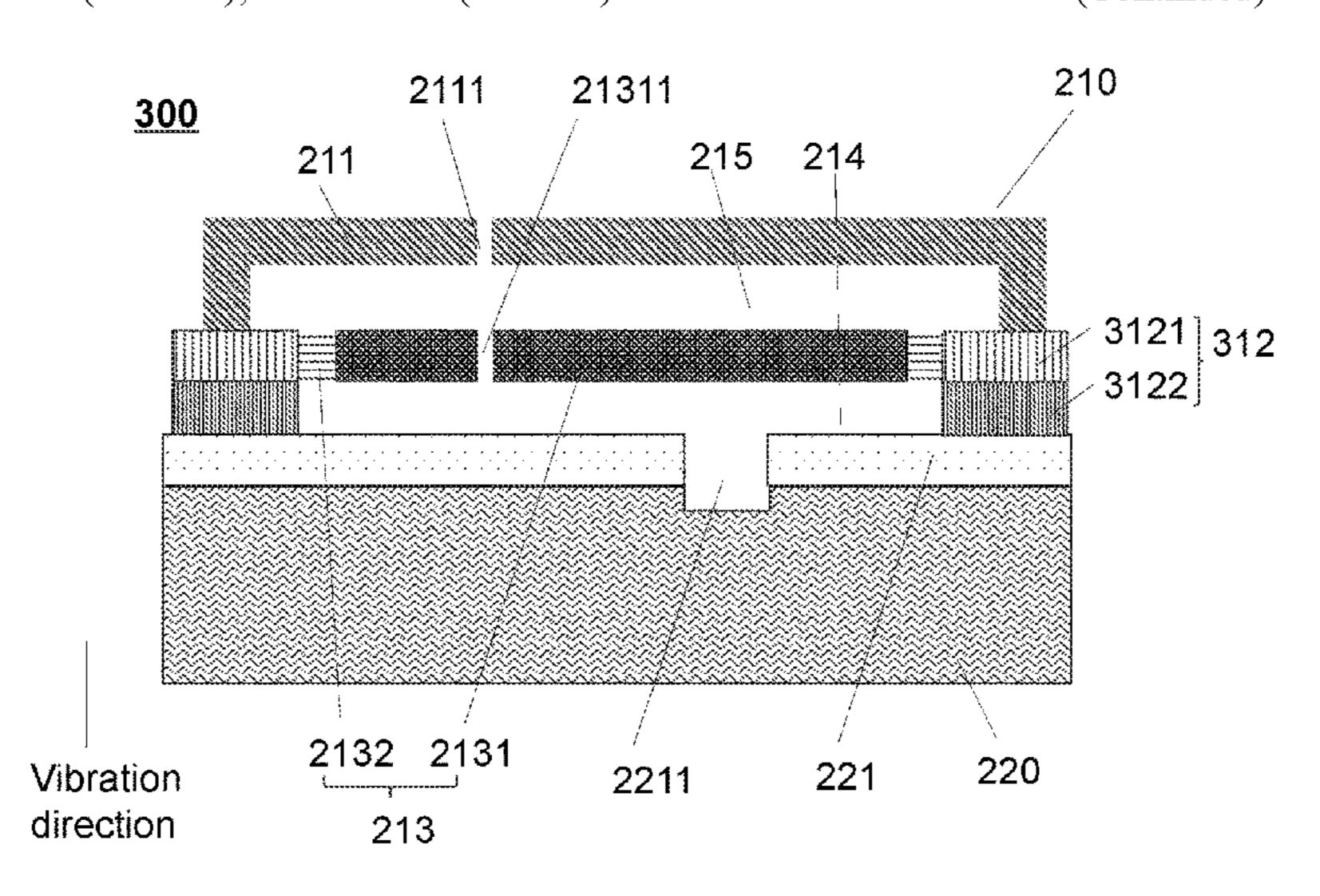
a mass element and an elastic element. A first side of the elastic element may be connected around a side wall of the mass element. A second side of the elastic element may be connected with the limiter.
