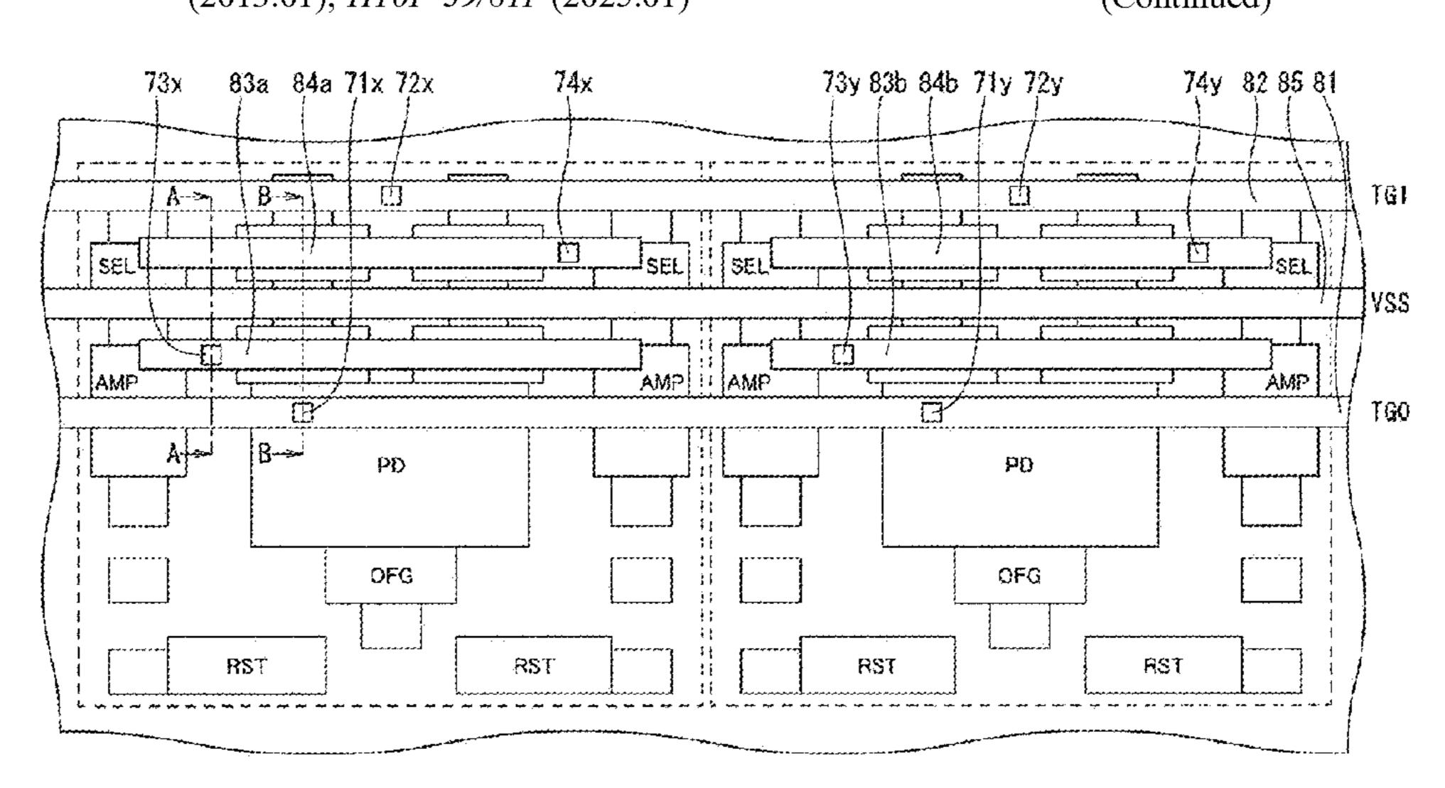
transistor of each of the pixels in the same row extends in a row direction in a first wiring layer, and the connection wiring extends to the first wiring layer.
