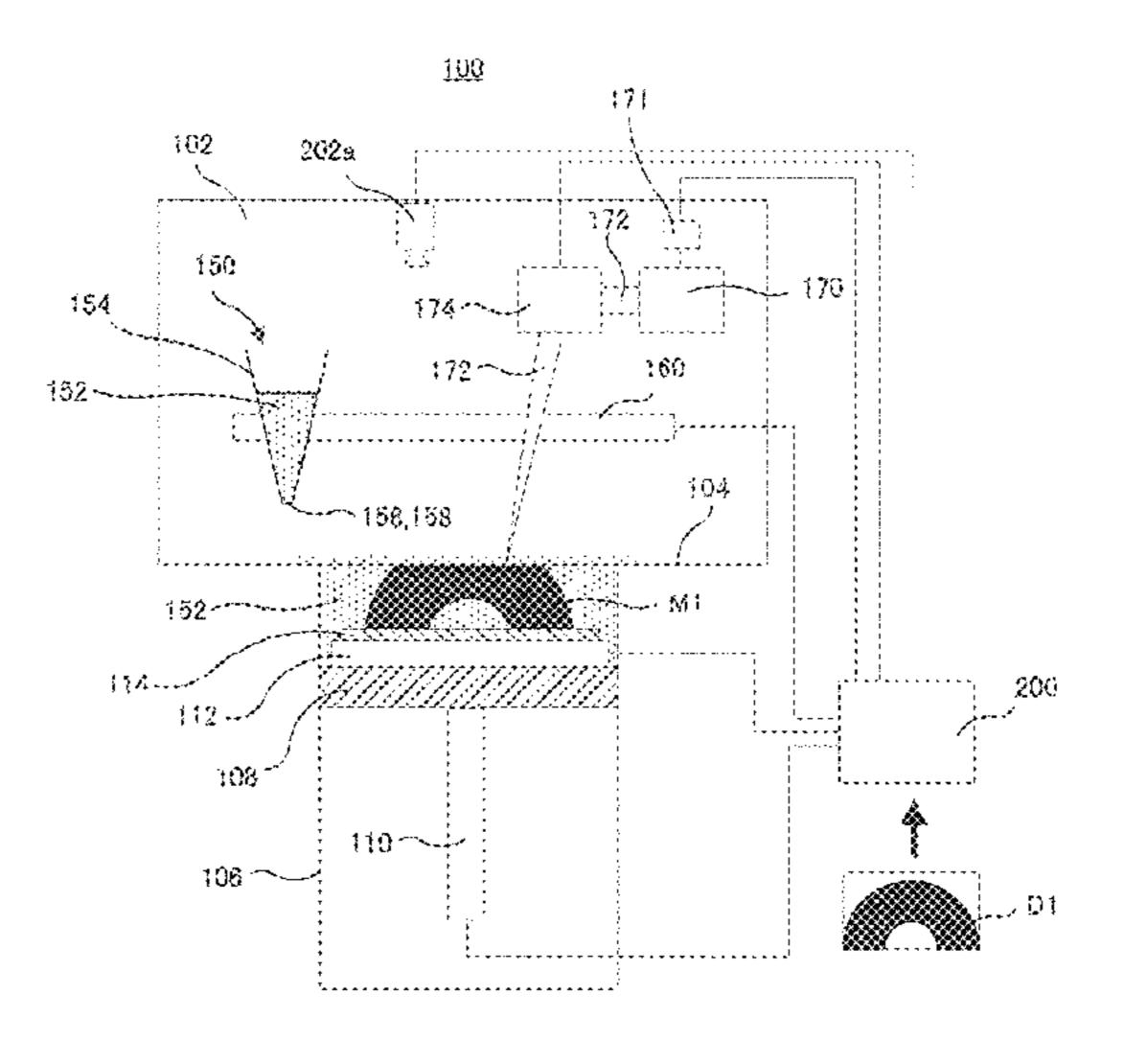
the determined irradiation position, a detector configured to detect an irradiation position of the beam applied into the chamber, and an evaluator configured to compare the determined irradiation position and the detected irradiation position.
