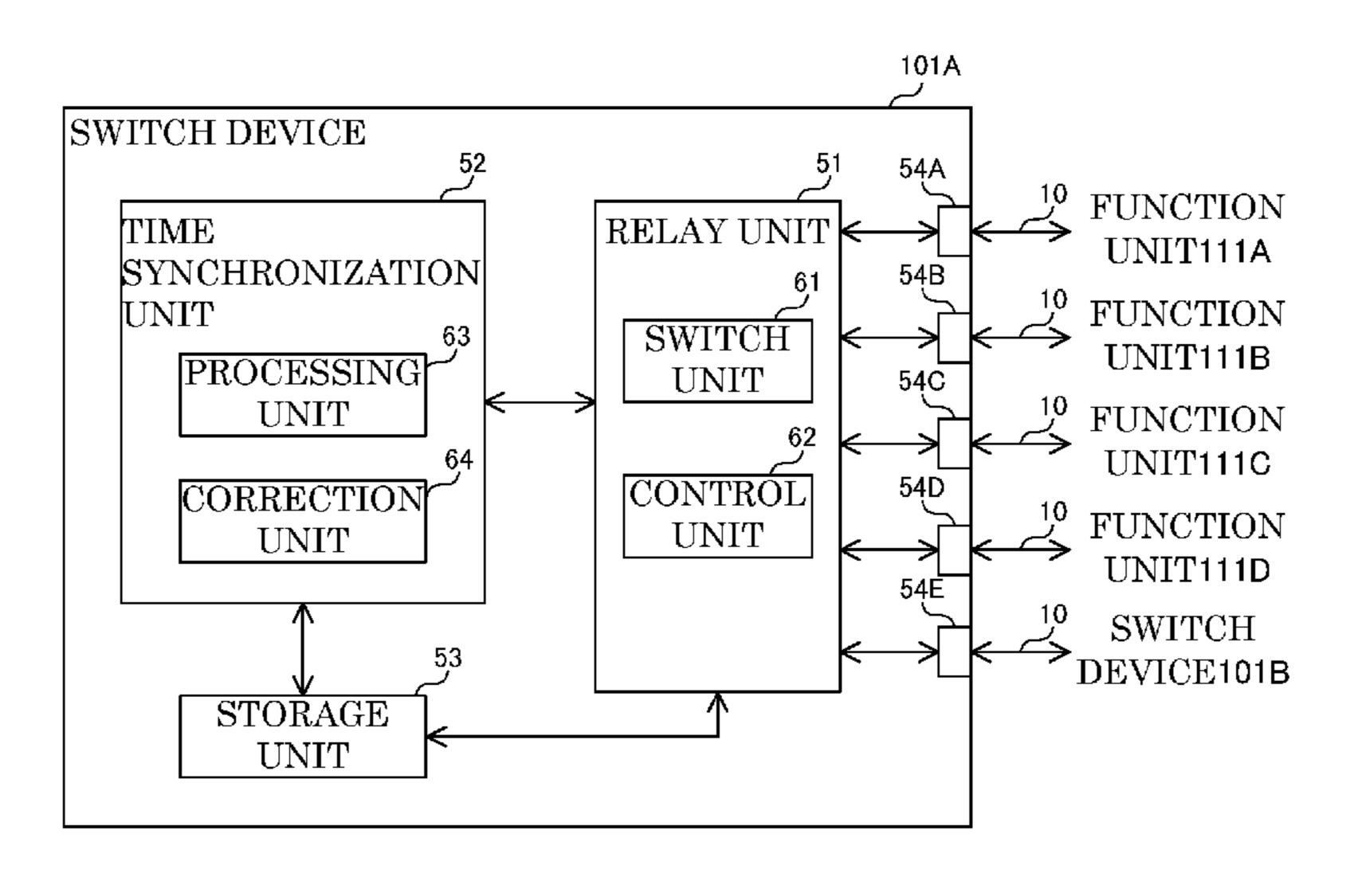
the other device. A propagation delay time between the devices is measured by time synchronization information to and from the other device, the measured propagation delay time is corrected based on the stored delay time information, and time synchronization between the devices is performed.
