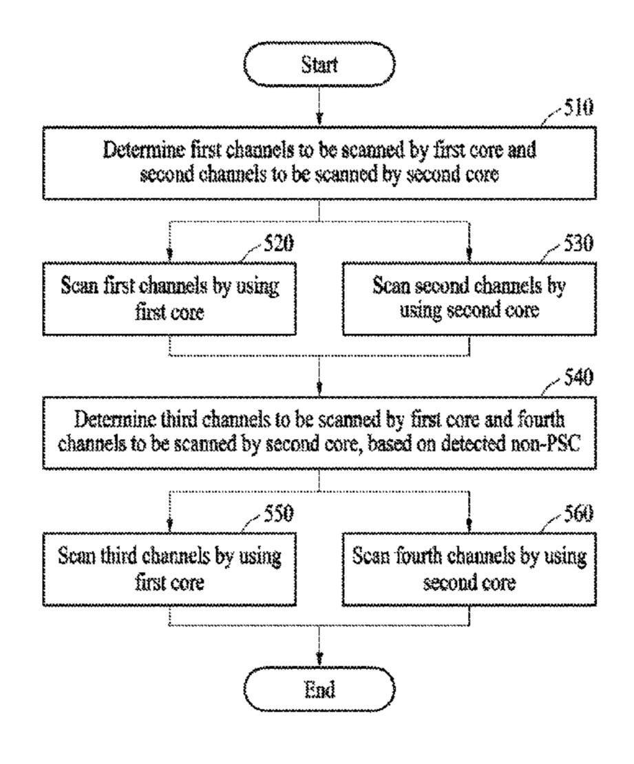
channels by using the first core, and scan the fourth channels by using the second core.
