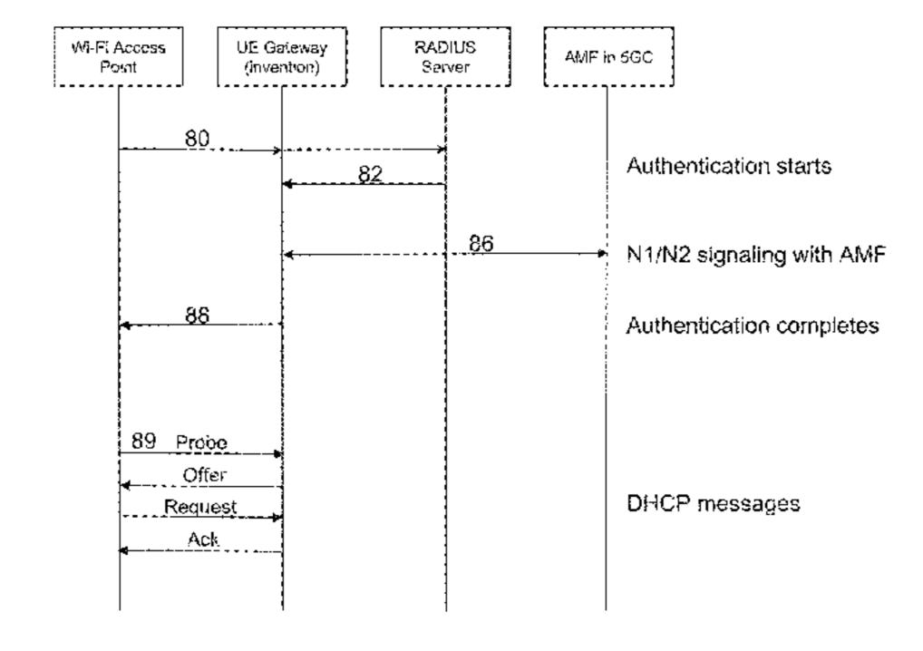
After above messaging, data packets travel between device and UPF of the 5G Core (via Wi-Fi Access Point and UE Gateway)
