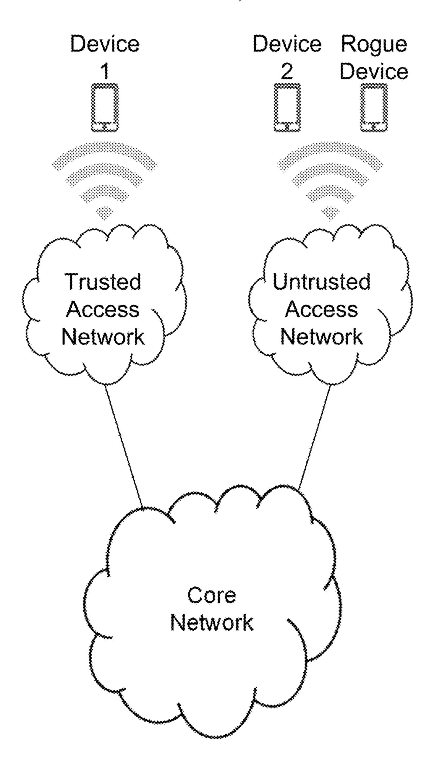
Figure 9. Trusted and Untrusted Access Networks
