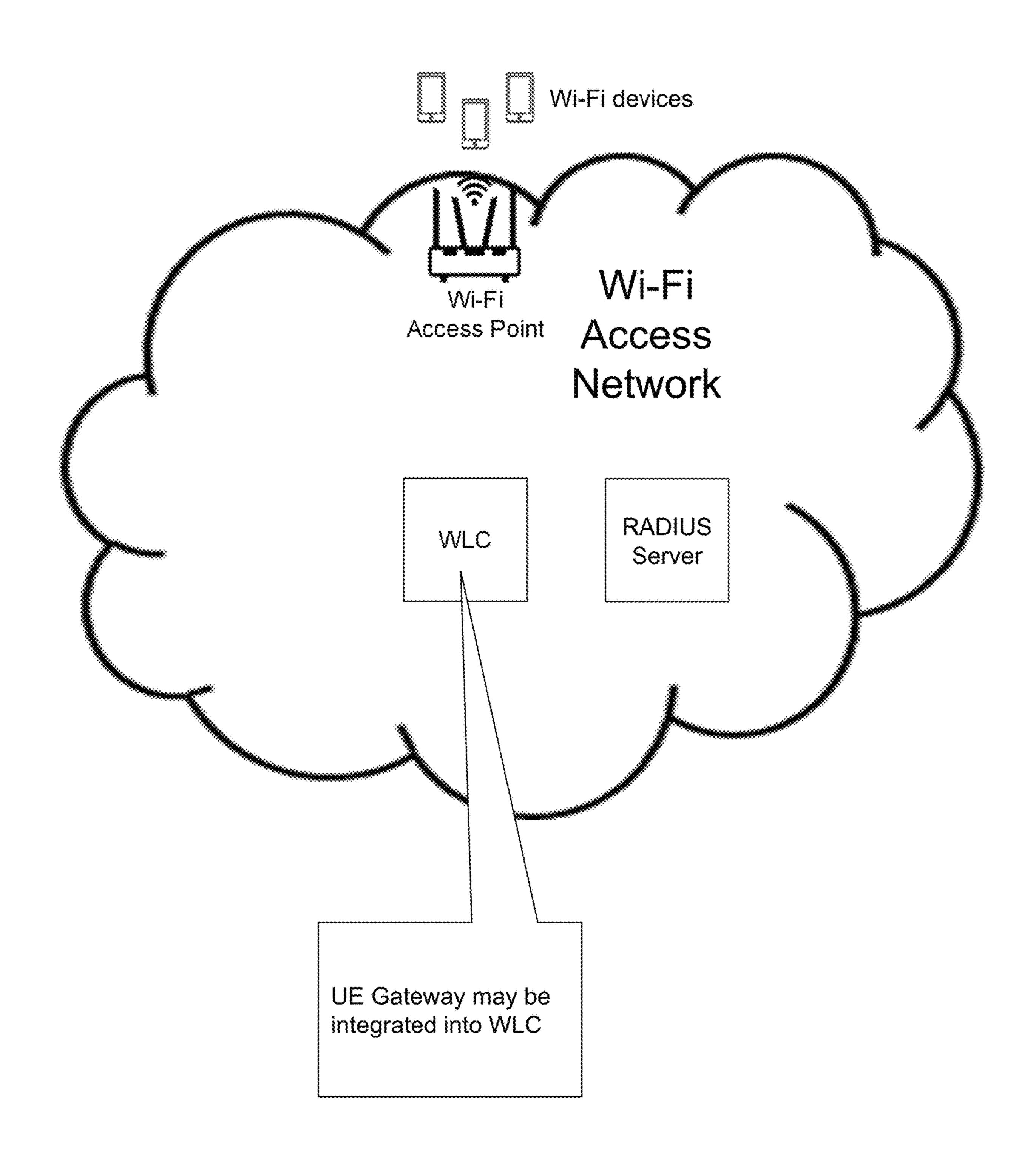
Figure 7. Wi-Fi Access Network
