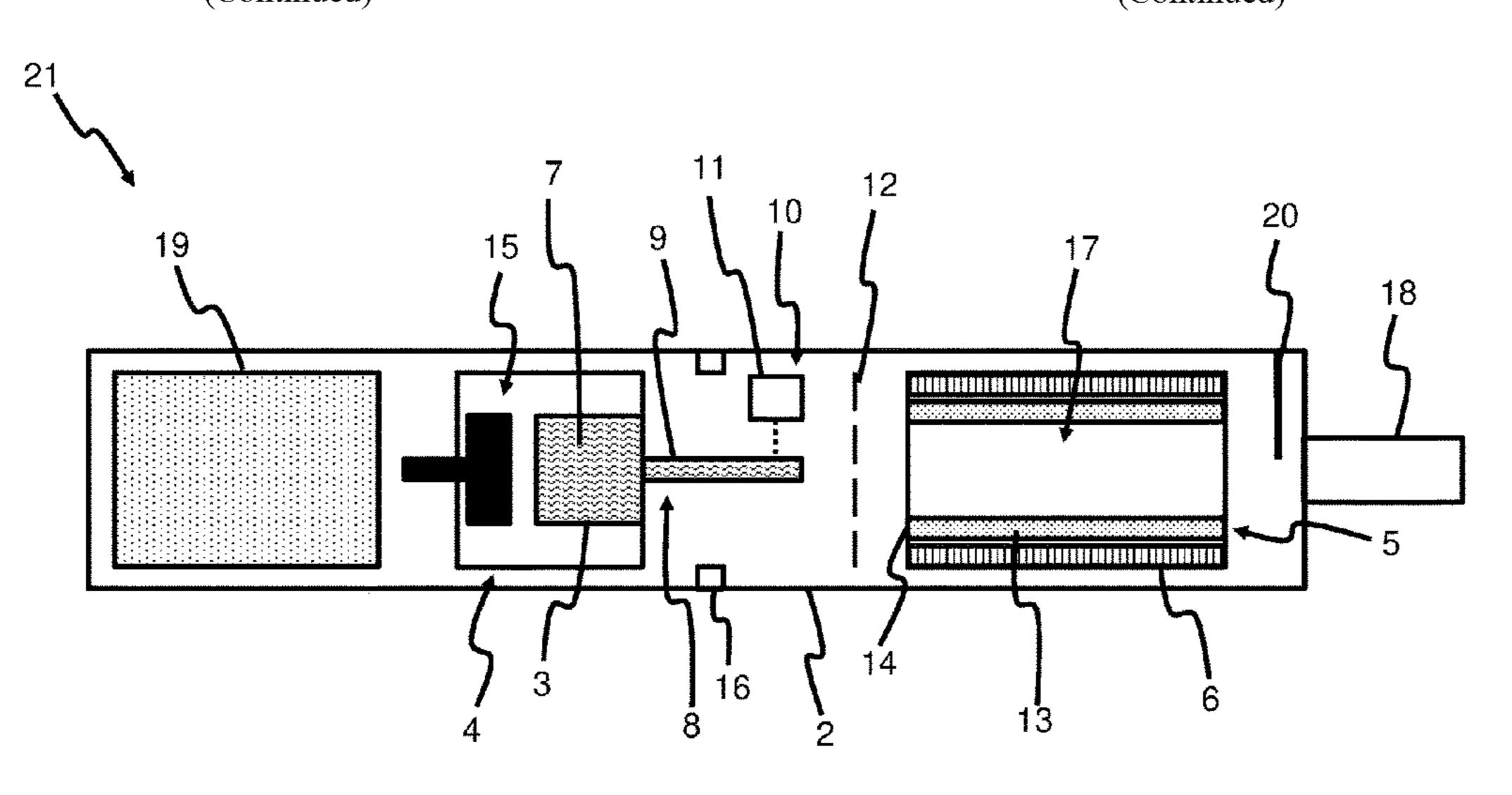
circuit ground; a second storage portion; a second liquid aerosol-forming substrate contained within the second storage portion; a heater to heat second liquid aerosol-forming substrate from the second storage portion; and a mixing chamber in fluid communication with the nozzle and the heater, the heater being downstream of the nozzle. A method of generating a mixed aerosol by the aerosol-generating device is also provided.
