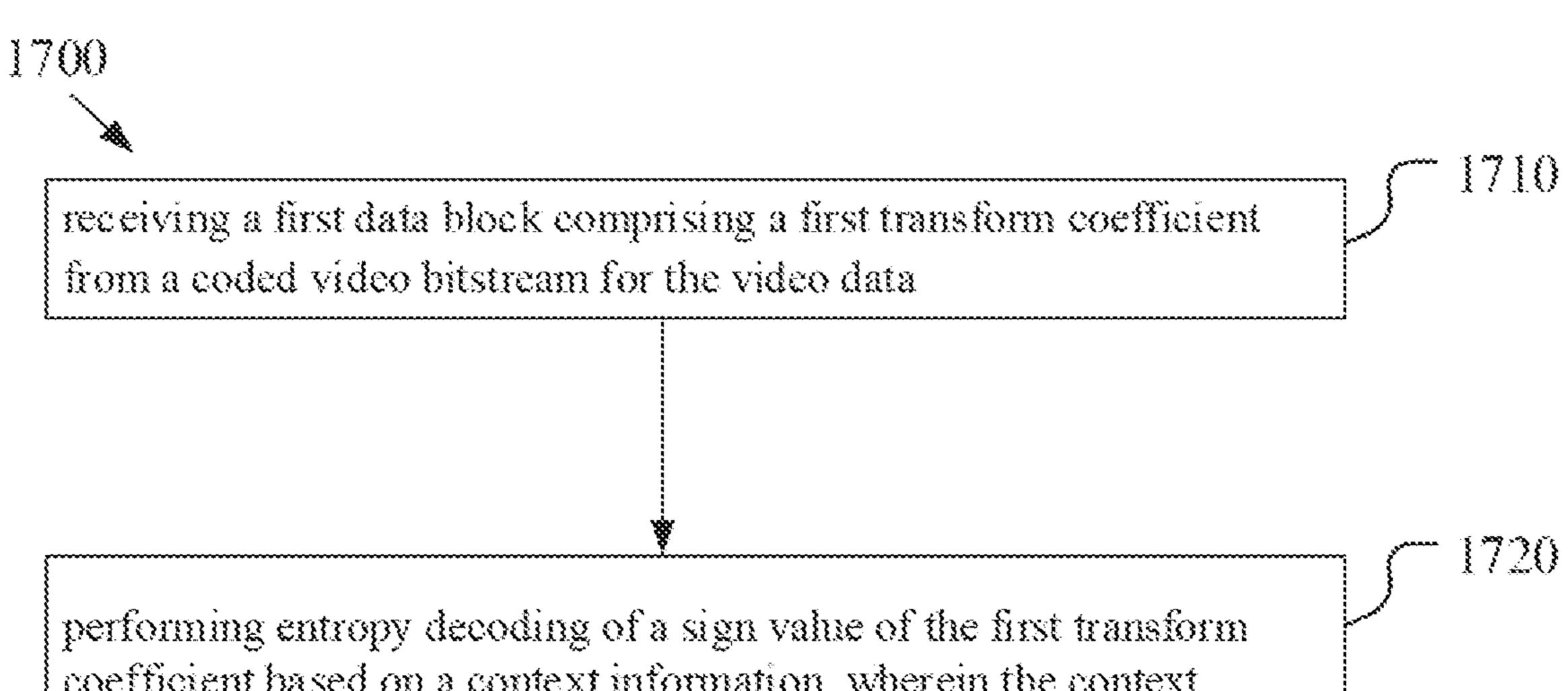
coefficient based on a context information, wherein the context information is derived based on a sign value of a second transform coefficient in a second data block in the video data, the second data block being co-located with the first data block, wherein co-located refers to two data blocks in different channels being located in a same spatial position.
