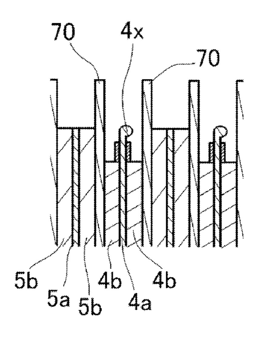
electrode core body in the thickness direction of the positive electrode core body, whereas the other surface of the positive electrode core body has no protrusion formed to protrude from said other surface of the positive electrode core body in the thickness direction of the positive electrode core body.
