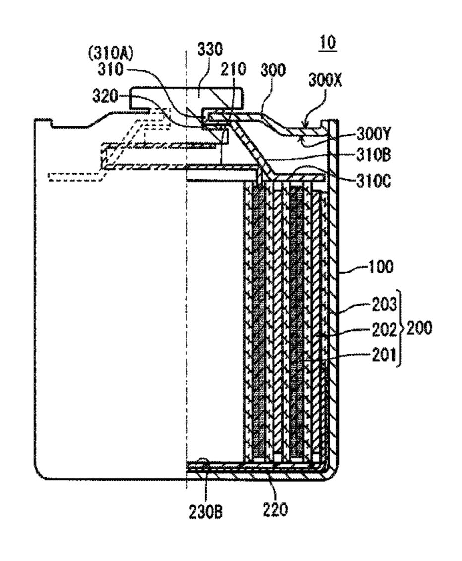
recessed in a periphery of the plate part in the radial direction. The internal lead is partially disposed in the cut-away portion.
