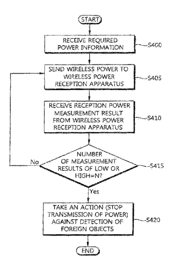
ratus are recognized, and a user removes the foreign objects. Accordingly, damage to a device attributable to foreign objects can be prevented.
