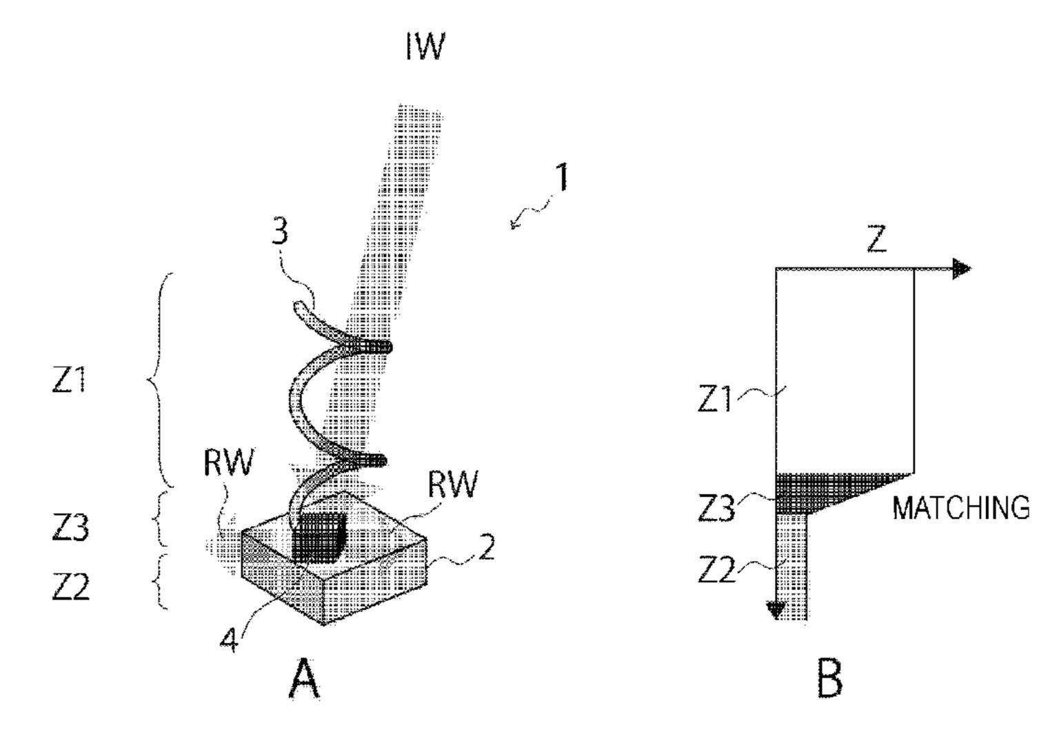
having the matching element 6 disposed between the base 2 and the spiral part 3 to moderate a change in the entire impedance value.
