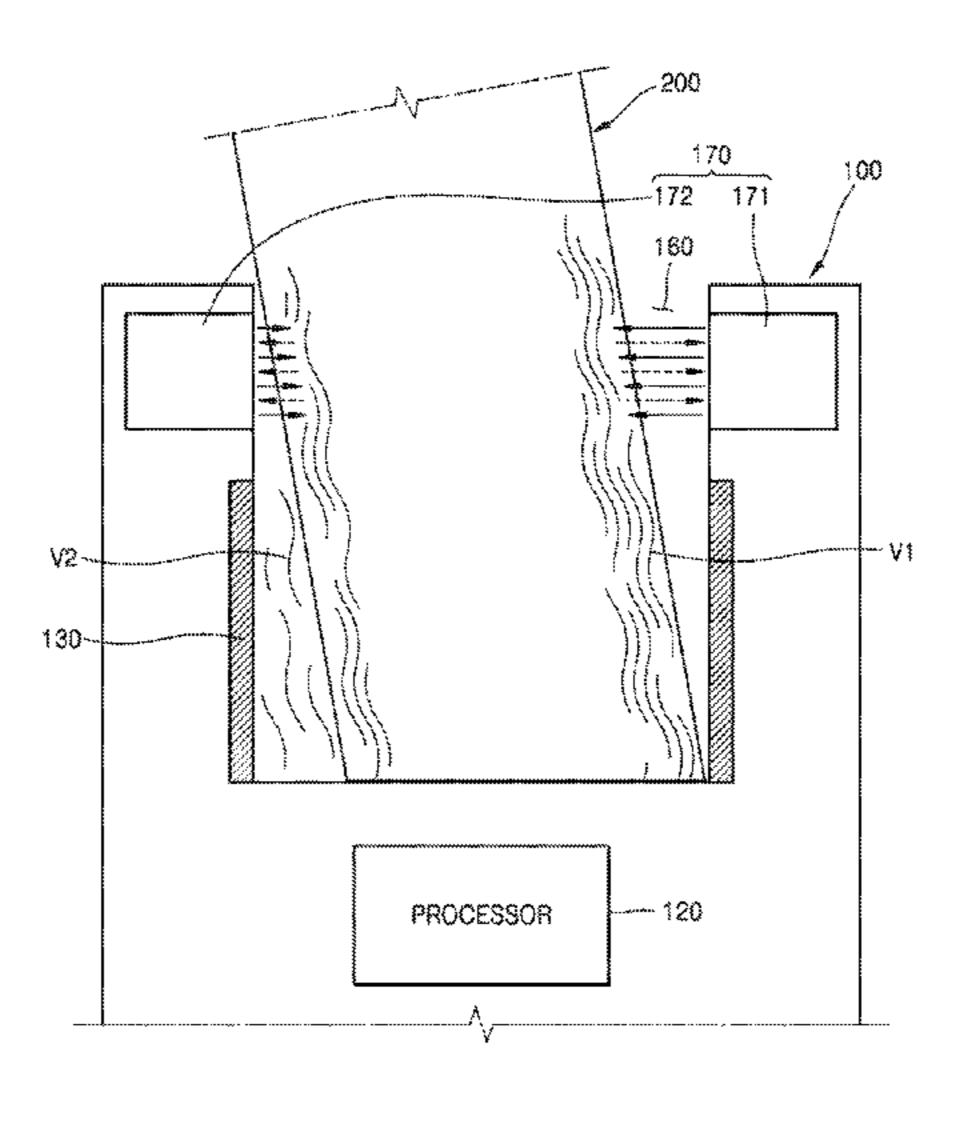
ated by the transducer, and control an operation of the heater based on the determined type of the aerosol-generating article.
