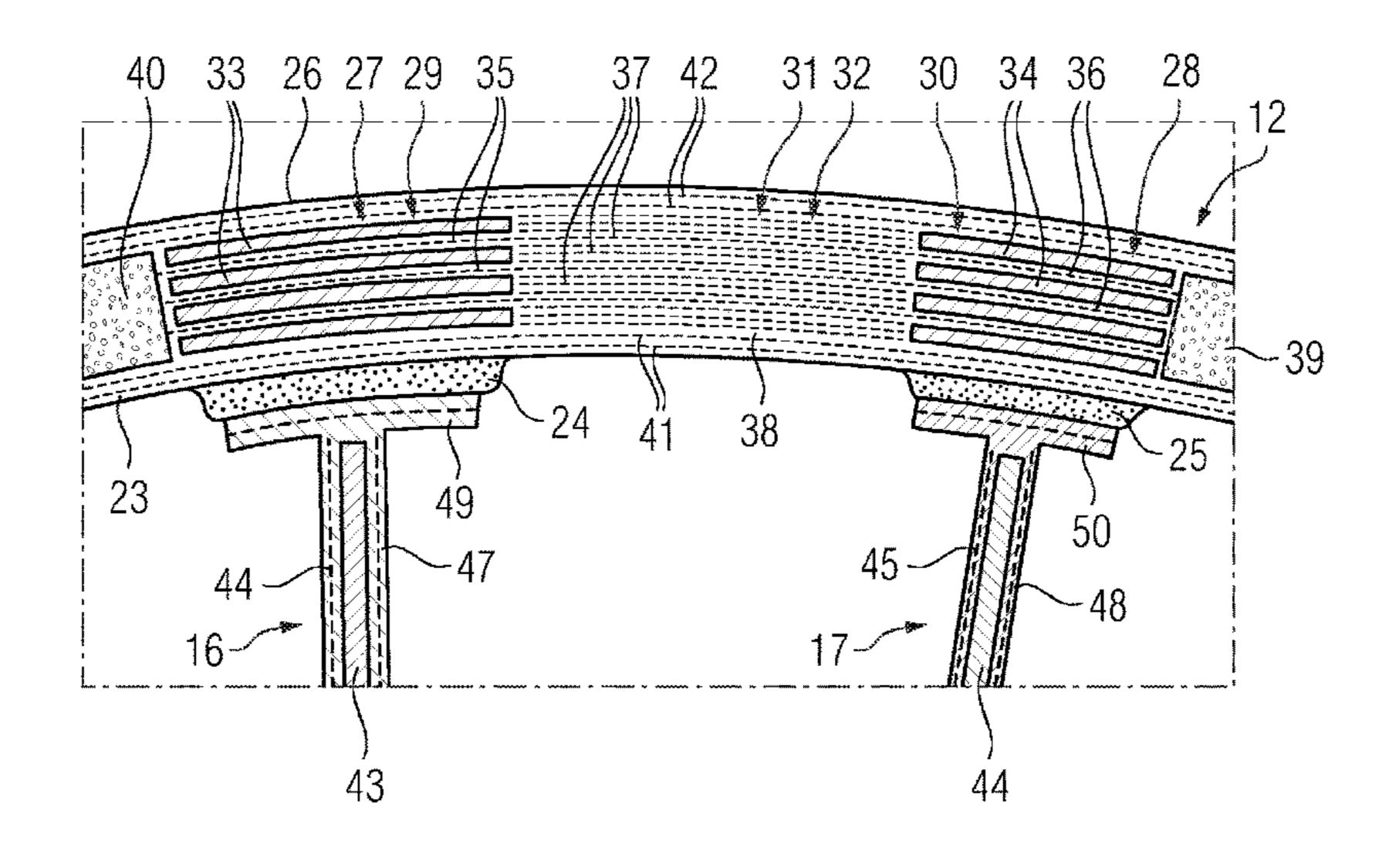
reinforcement structures over at least a part of their length comprising at least one stack composed of several glass fiber layers infused with resin is arranged between the reinforcement structures.
