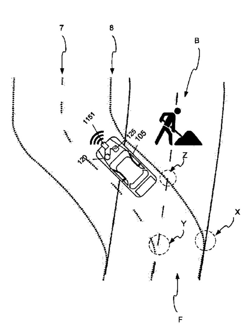
the result of the checking is that there is a motorway exit or roadworks on the first side of the vehicle and that the environment sensor system detects the lane marking, operating a lane-keeping function of the driver assistance system; and if the result of the checking is that there is a motorway exit or roadworks on the first side of the vehicle and that the environment sensor system does not detect the lane marking, triggering a takeover request to a driver of the vehicle.
