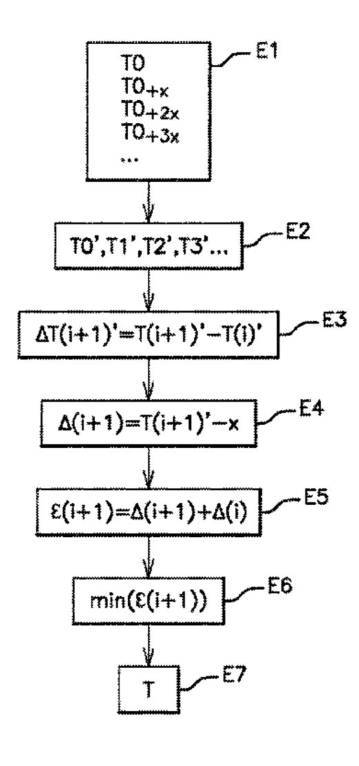
sisting in summing the discrepancy calculated for a time value received at one instant and a time value received at the previous instant; determining the actual time for adjusting the on-board clock according to the disparity.
