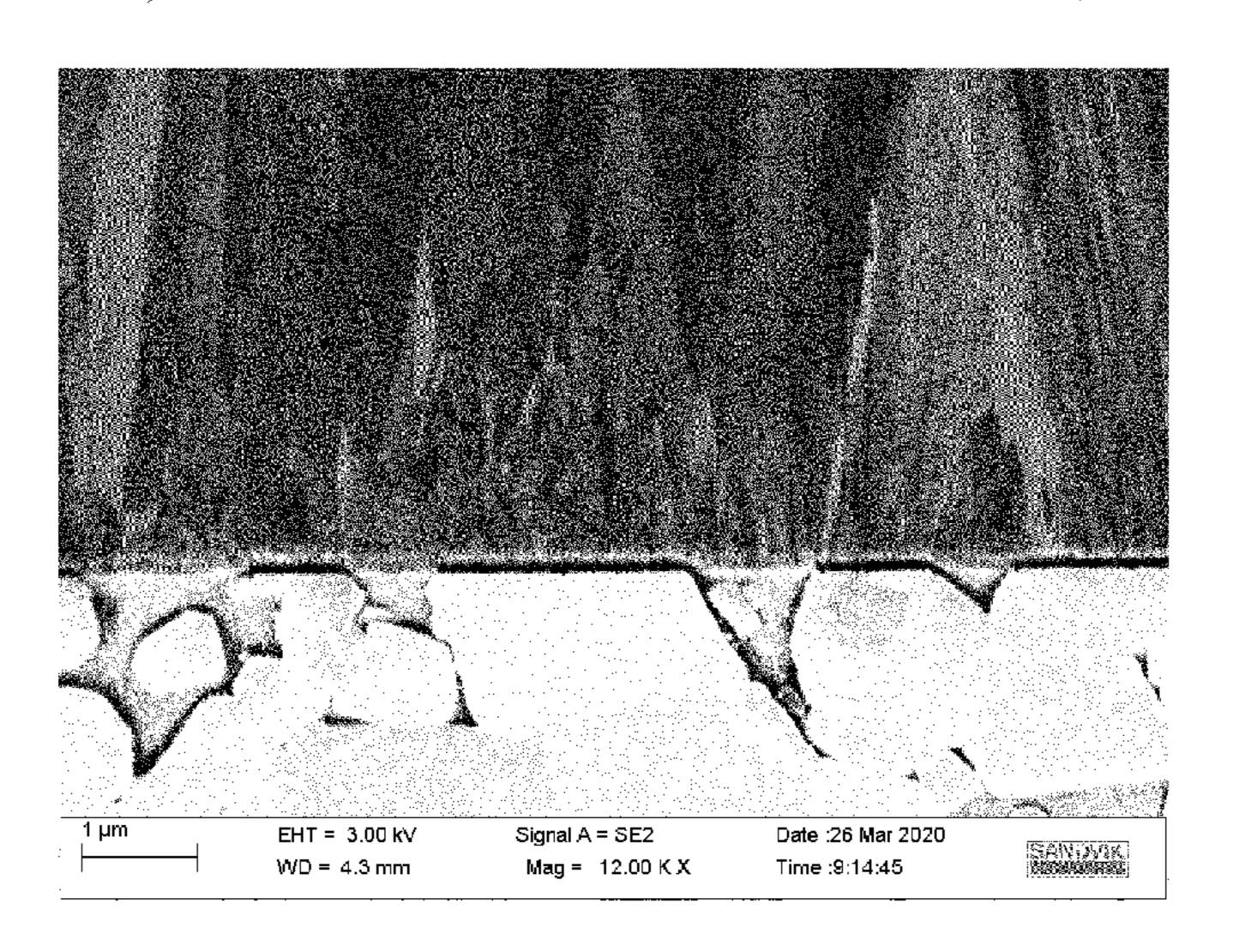
inner layer of TiN and a subsequent layer of TiCN. A C-activity relative to graphite in the metallic binder is lower than 0.15 and an average d electron value of the metallic binder is 7.00-7.43, wherein an interface between the substrate and the inner TiN layer is free of Ti-containing intermetallic phase.
