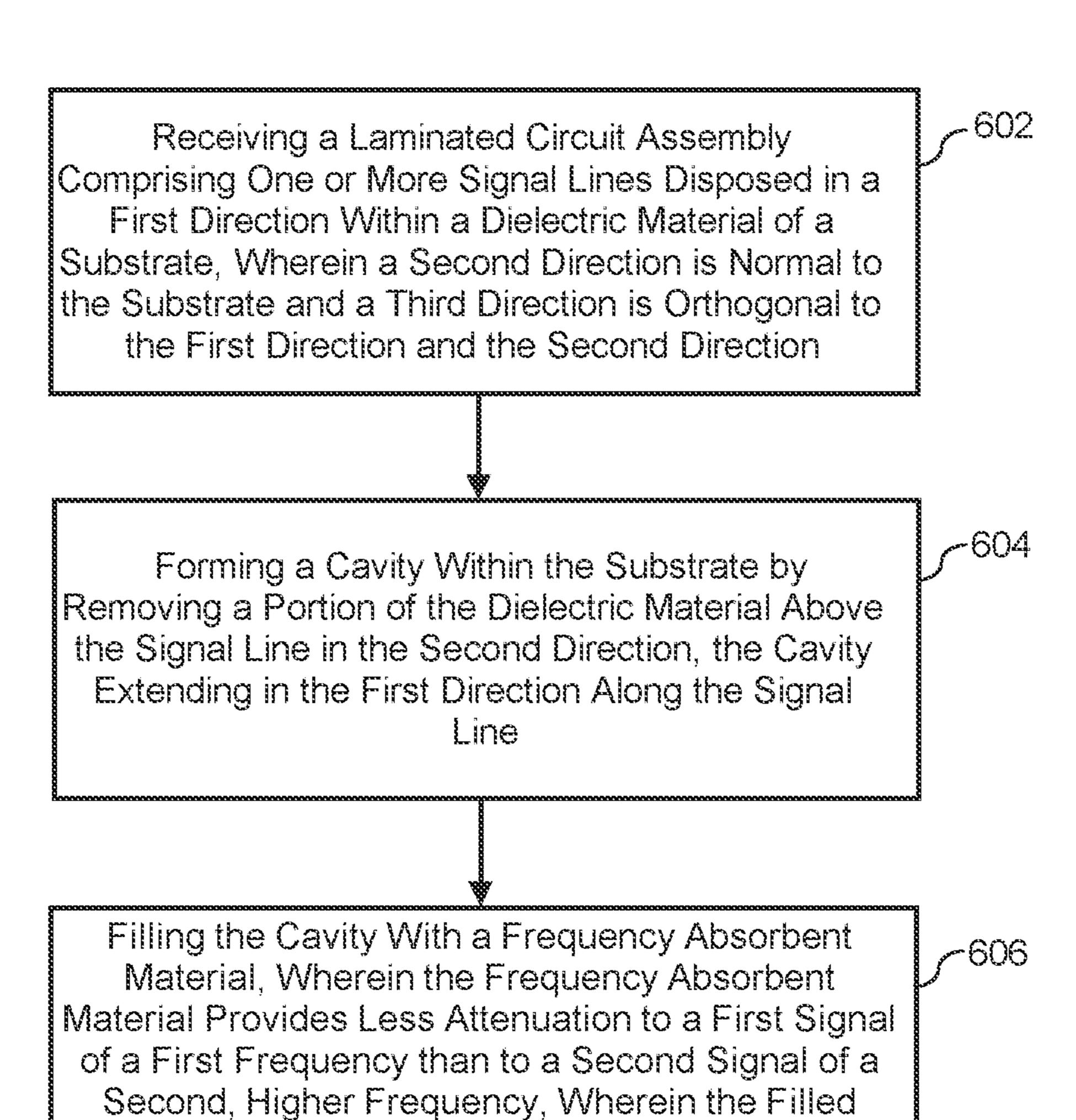
Cavity is Configured to Attenuate Infrared Signals
