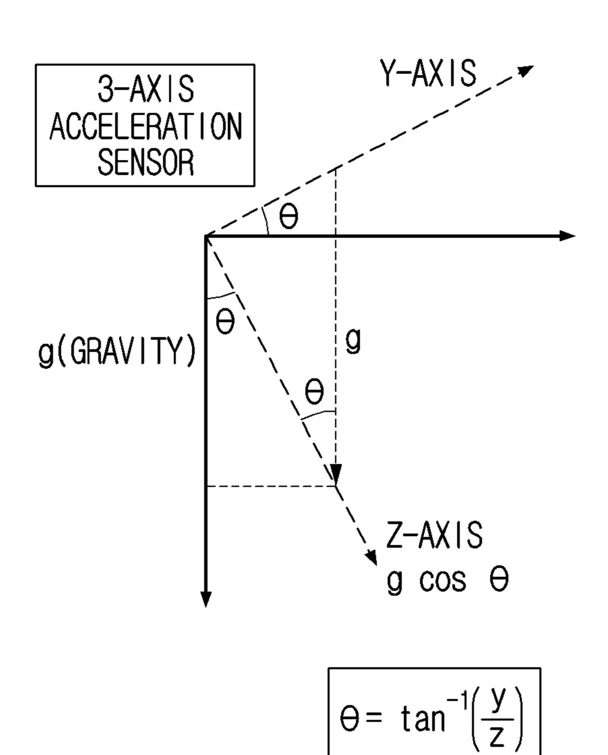
y: Y OUTPUT VALUE OF ACCELERATION SENSOR z: Z OUTPUT VALUE OF ACCELERATION SENSOR
