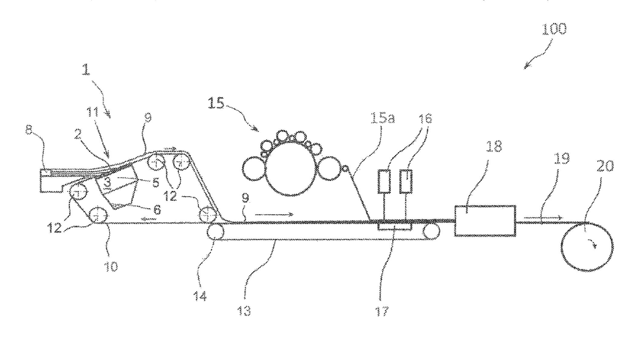
ured to introduce a roller card web into the installation, a hydroentanglement arranged downstream in the material transport direction and including at least one water beam configured to entangle, bond and/or structure a single sheet of fibres or a plurality of sheets of fibres, and a dryer arranged downstream in the material transport direction.
