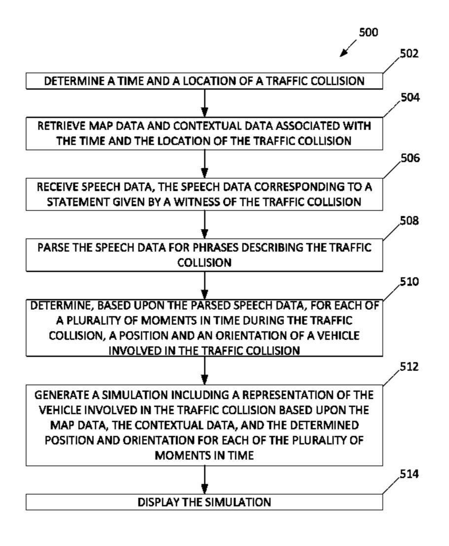
simulation of the traffic collision including a representation of the AV based upon the map data, the contextual data, and the vehicle telematics data, and provide content to enable display of the simulation on a display device.
