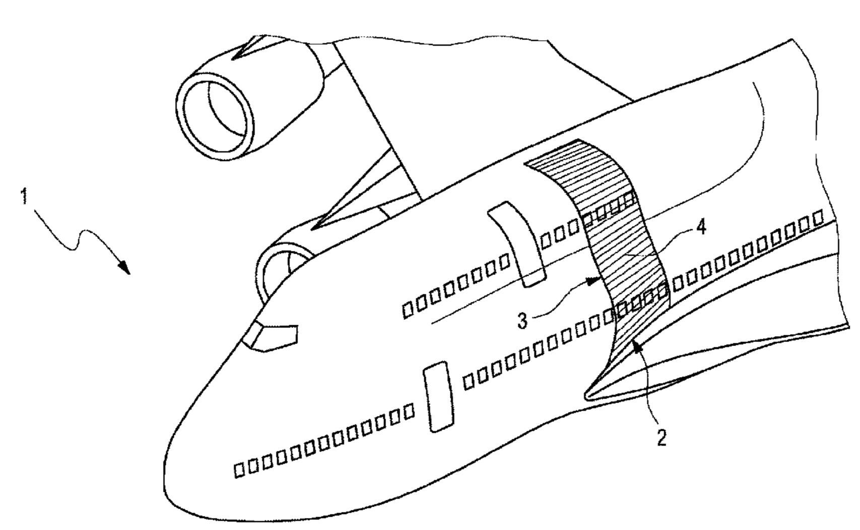
flow direction of the respective field; and applying the aerodynamically functional film to the body within the field boundary of the at least one field located in the developed surface segment in such a way that the aerodynamically functional film is aligned along the main flow direction of the respective field.
