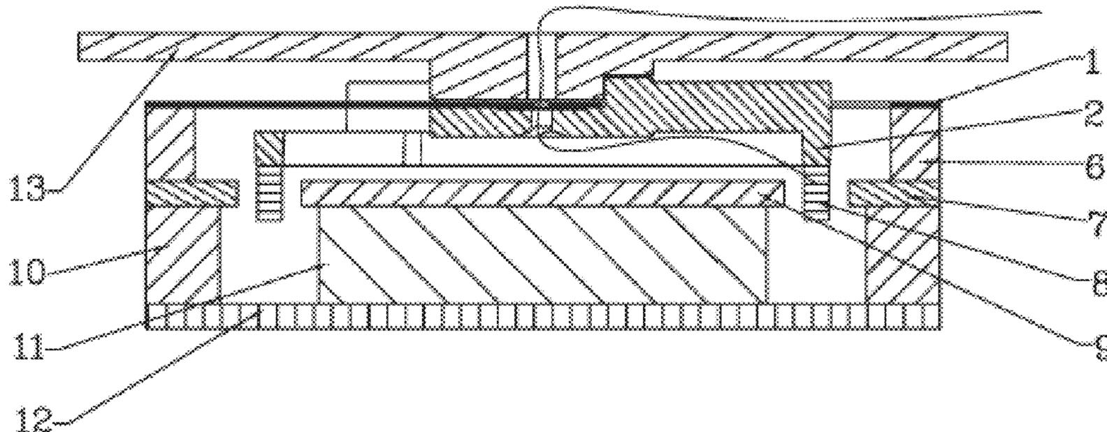
torus comprises a fixed voice coil, which is driven by the magnetic system. The bone conduction speaker in the present disclosure and its compound vibration device adopt the fixed vibration conductive plate and vibration board, making the technique simpler with a lower cost; because the two adjustable parts in the compound vibration device can adjust both low frequency and high frequency area, the frequency response obtained is flatter and the sound is broader.
