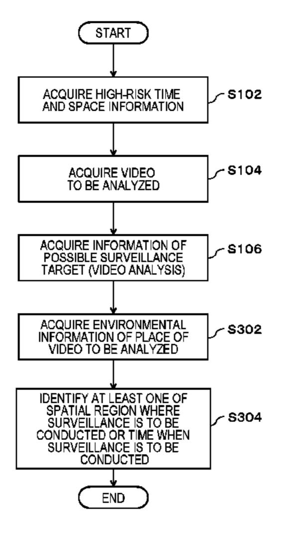
time and space identification unit (130) that identifies at least one of a spatial region where surveillance is to be conducted which is at least a portion of the spatial region or a time slot when surveillance is to be conducted, from among the spatial region and the time slot indicated by the high-risk time and space information, on the basis of the information of the possible surveillance target.
