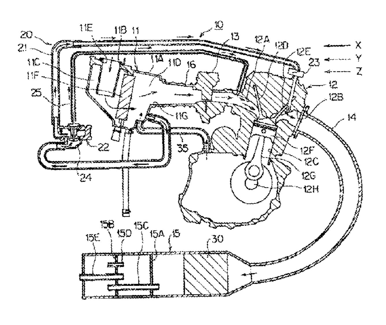
an exhaust gas flow path, and a catalyst layer provided on a surface forming the flow path of the metal foil, wherein the catalyst layer contains a noble metal, an OSC material containing cerium and a rare earth element other than cerium (non-Ce rare earth element), and alumina, and a content of the non-Ce rare earth element with respect to 100% by mass of the catalyst layer is 2.52% by mass or more and 4.62% by mass or less in terms of an oxide.
